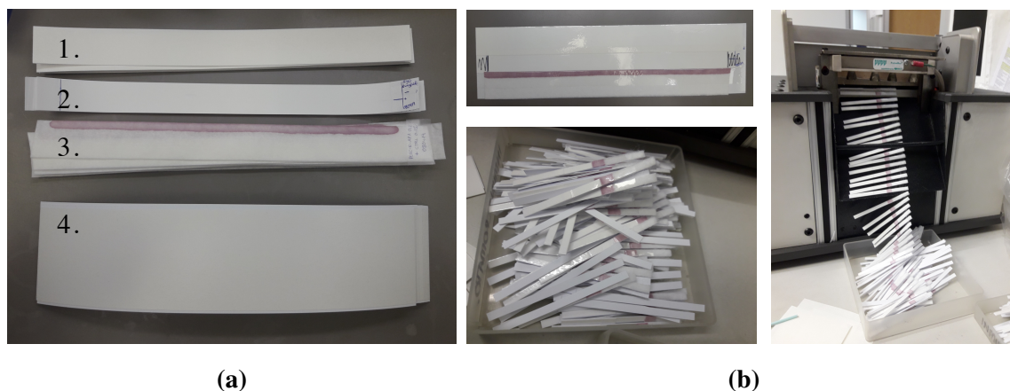
Figure 5.7: Manufacturing process of CCHFV NP-specific LFA tests. (a) Picture showing the different components used for the fabrication of the CCHFV NP-specific LFAs: 1. absorbent pad, 2. nitrocellulose membranes, 3. conjugate pads and 4. adhesive cards. (b) Pictures of a fully assembled LFA cardboard (top left), strips cutting process (right) and ready-to-use LFA strips (bottom left).
