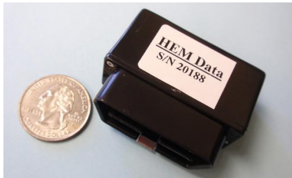
Figure 3.4 Photograph of the HEM OBD mini-logger. Source: HEM Data (2020).
