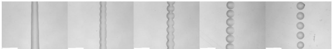
Figure 56 - Deposition of PDMS droplets with decreasing spacing. All scale bars are 500 \mu m.
