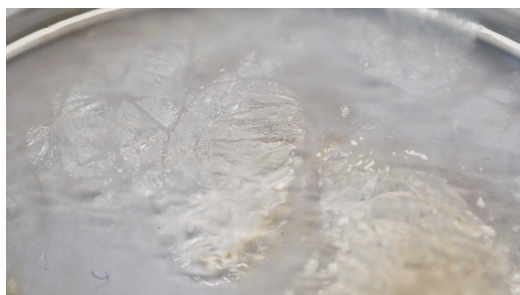
Figure 45 - Skin curing of DMS-V21 through exposure to deep UV
