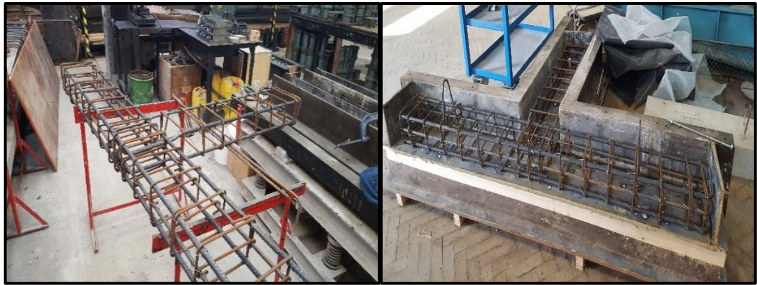
Figure 3.20: Reinforcements detailing the beam-column joints
