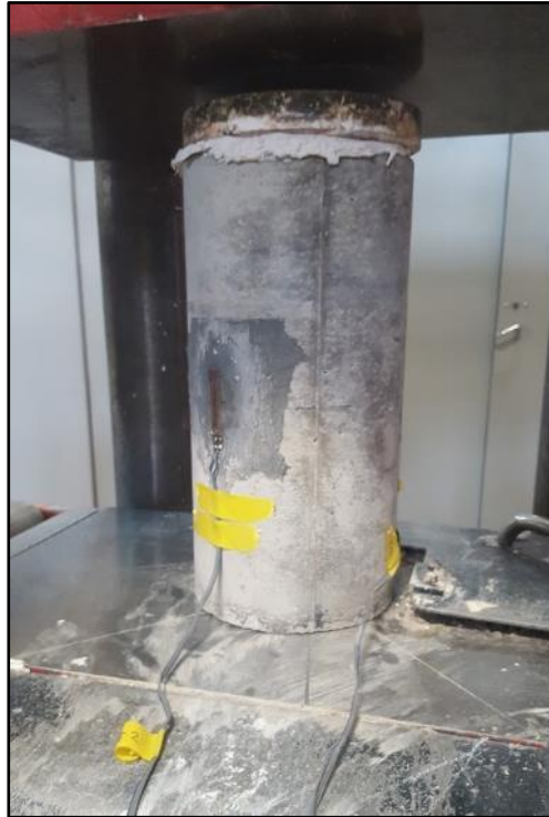
Figure 3.11: Test of modulus of elasticity
