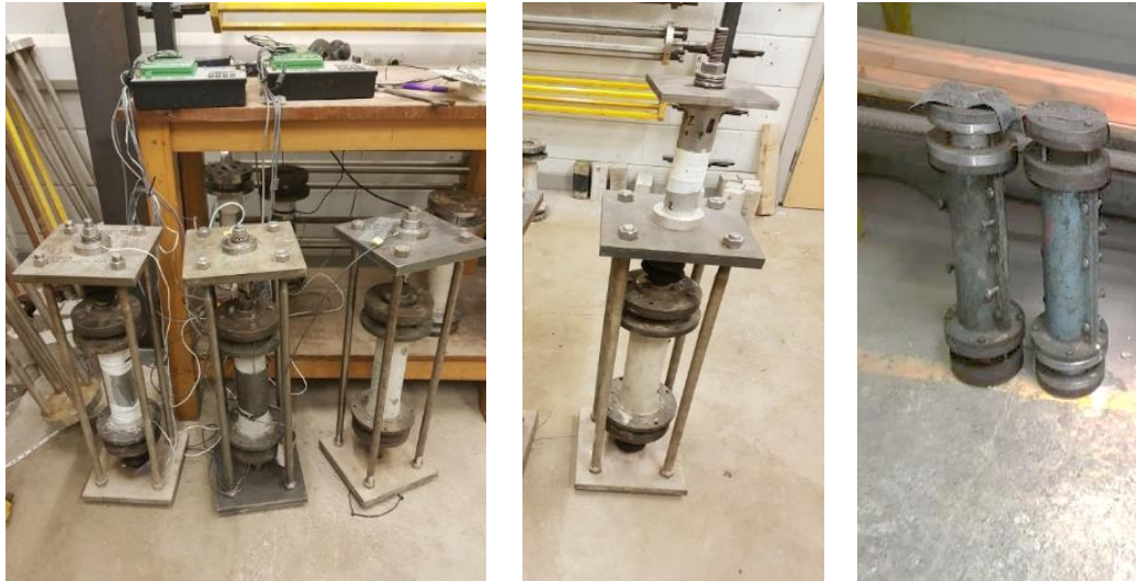
Figure 3.15: Tensile creep test
