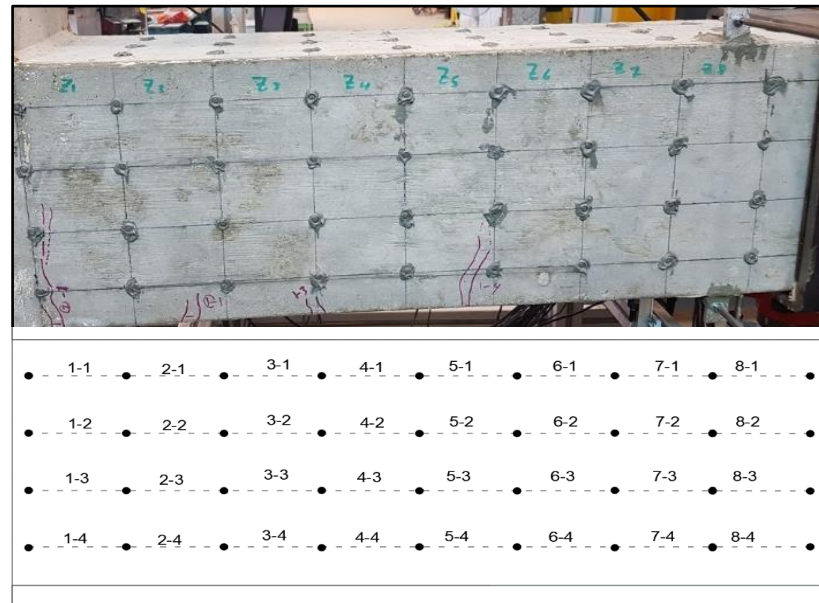
Figure 3.29: DEMEC points on the beam's sides
