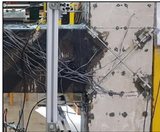
Figure 3.28: a) Schematic diagram of the joint deformation b) Diagonal LVDT's
