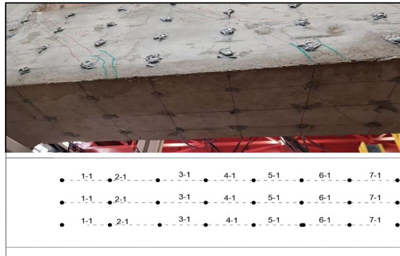
Figure 3.30: DEMEC points on the beam's bottom and top
