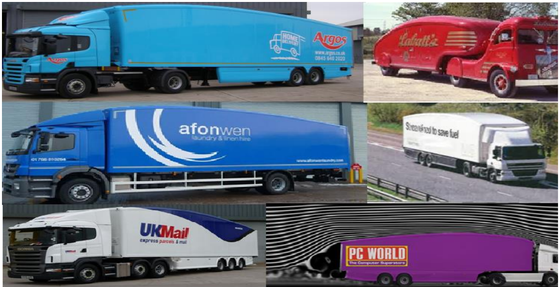
Fig. 3.27. Examples showing contemporary curved roof sections of HGV compared to the Labatt's streamliner from 1947 (Cooper, 2004, De Boer et al., 2016).
