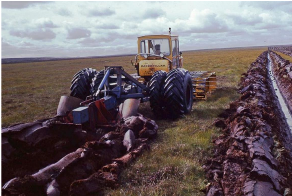
Figure 1.2. Preparation of peat ridges for planting in 1979 using a double mould board plough mounted on a low ground pressure tractor at Rumster Forest, Caithness. Bad a'Cheo forms part of the wider Rumster Forest area, and although planted earlier it would have been prepared in a similar manner. Photograph by George Day, sourced from the Forestry Memories Image Library, https://www.forestry-memories.org.uk/ .
