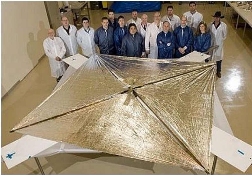
Figure 2.5: NanoSail-D2 ground deployment test. www.nasa.gov
