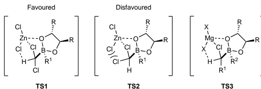
**Figure 11:** Transition states to explain the stereoselectivity of the Matterson homologation.<sup>72,73</sup>
