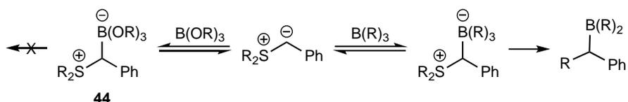
**Figure 12:** Reversibility of boron 'ate' species produced from lithiated sulphur ylides. Alkyl boranes undergo 1,2-metallate rearrangement whereas boronic esters do not.
