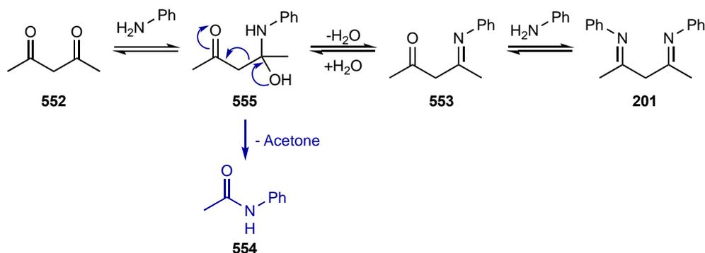
**Figure 26:** Simplified route to the formation of 1,3-diketimine **201** and acetanilide **554**.
