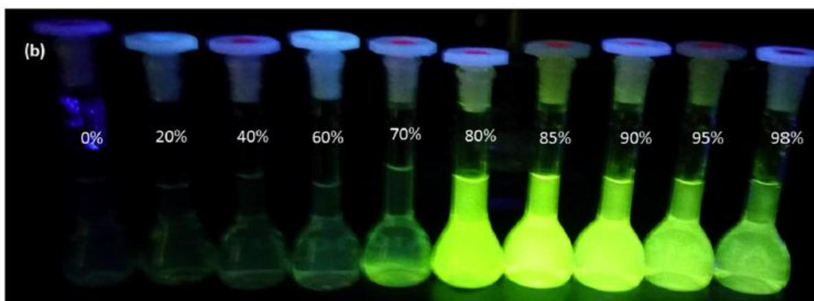
**Figure 2. 12.** The fluorescence emission of Probe 1 (20  $\mu$ M) in mixtures of H<sub>2</sub>O/THF with increasing water fractions [105].
