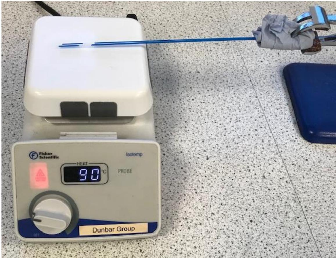
*Figure 4. 3. Wet stripped optical fibre sections drying near the hot plate surface set to 90 °C.*
