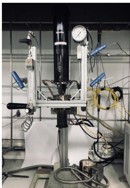
The reaction vessel for the liquefaction process. Cynthia Kartey, Author provided
