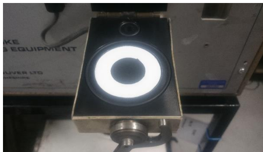
Figure 3.9 Filter paper in the electrically heat holder after collection of particles. The black circle indicates mainly soot particles. If the volatiles are high the circular spot is brown.
