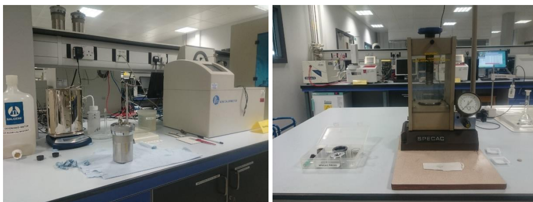
Figure 3.18 Bomb Calorimeter – Parr 6200.
