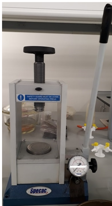
Fig. 3.2 This Specac Presser with a maximum pressure of 15 tons was used to compress the powdered sample and wax mix into pelleted solid discs.
