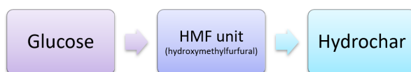
Fig. 2.10 A simple graphic demonstrating the relationship between the glucose molecule, the HMF unit and the hydrochar product, under hydrothermal conditions. Adapted from Kruse et al 2019 [135].
