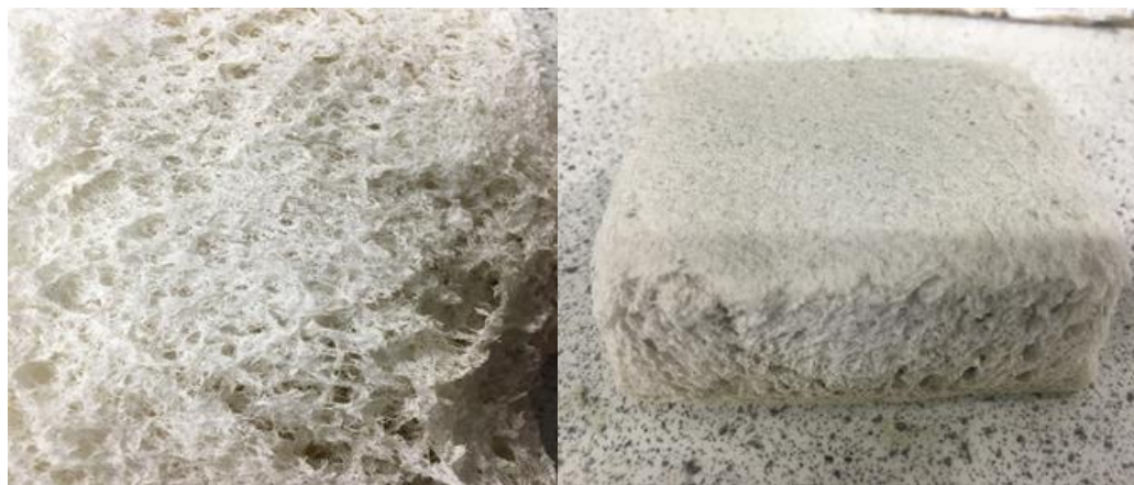
Figure 3. 50 Waste paper foam materials (3-Dimensional porous is displayed).
