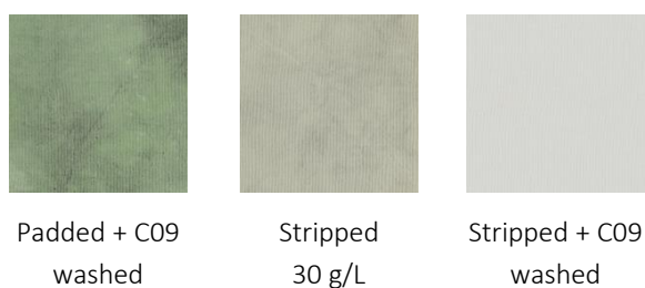
Figure 6.1 Visual appearance of PAE/pigment-padded cotton after padding and ISO 105 C09 washing (left), after stripping (middle) and after sequential stripping/C09 washing (right)
