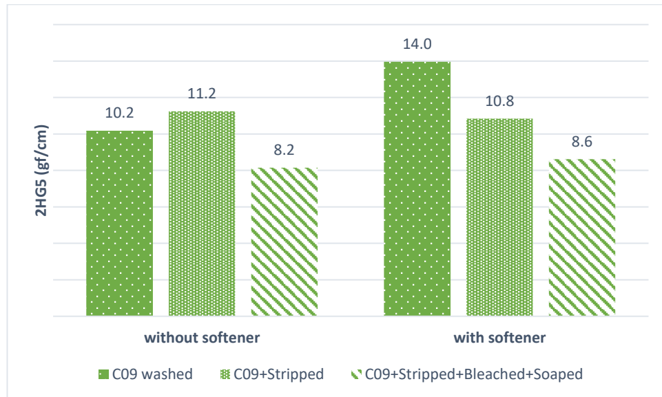
Figure 6.47 KES-F bending hysteresis 2HG5 for PAE/pigment-padded cotton fabrics with and without incorporation of a commercial cationic softener (Easy), stripped with 2.5 g/L Kybreak, from padding to sequential Kybreak stripping/bleaching/soaping
