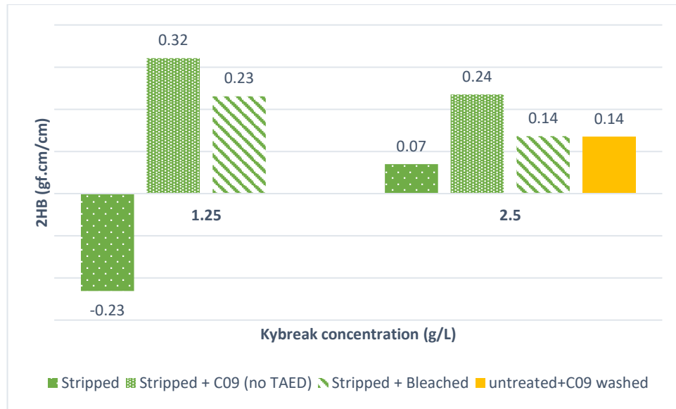
Figure 6.42 KES-F bending moment 2HB for fabrics stripped with 1.25 g/L and 2.5 g/L Kybreak, after stripping, after Kybreak stripping/C09(no TAED) and after Kybreak stripping/bleaching/soaping
