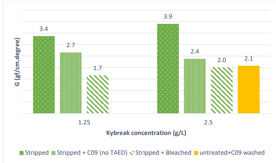
Figure 6.39 KES-F shear rigidity G for fabrics stripped with 1.25 g/L and 2.5 g/L Kybreak, after stripping, after stripping/C09(no TAED) and after stripping/bleaching/soaping, with untreated and ISO 105 C09 washed cotton fabric as a reference standard
