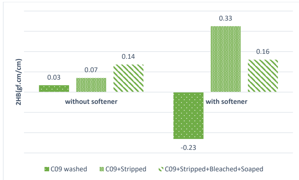
Figure 6.49 KES-F bending hysteresis 2HB for PAE/pigment-padded cotton fabrics with and without incorporation of a commercial cationic softener (Easy), stripped with 2.5 g/L Kybreak, from padding to sequential Kybreak stripping/bleaching/soaping
