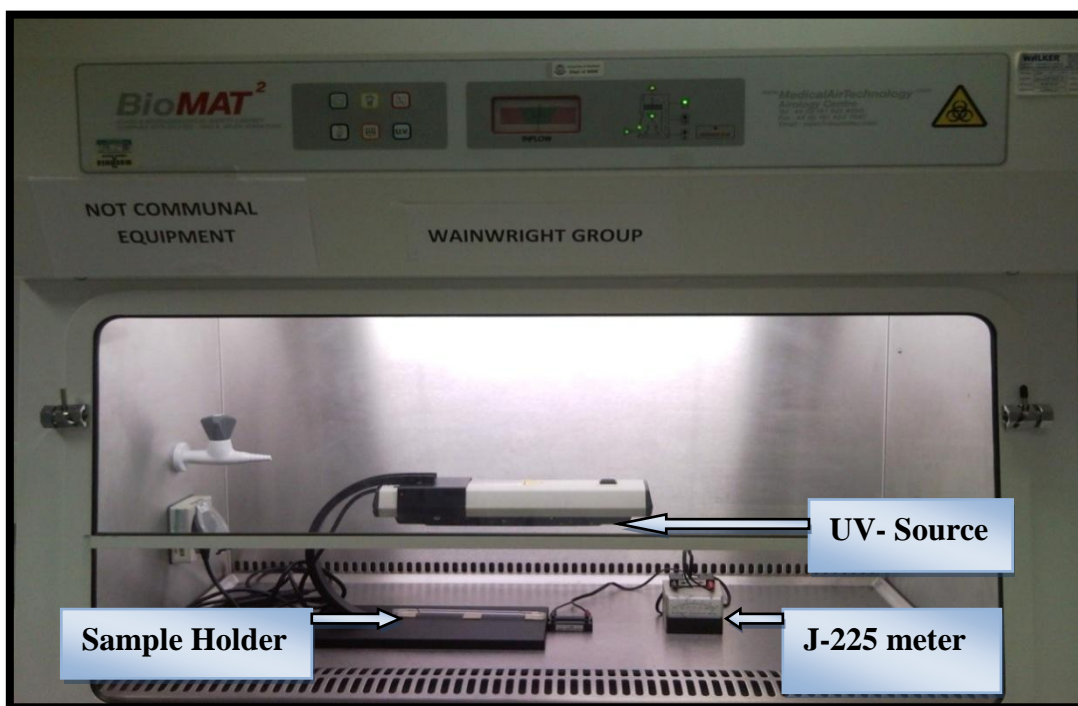
Figure 4.1: The UV exposure apparatus inside the laboratory hood.
