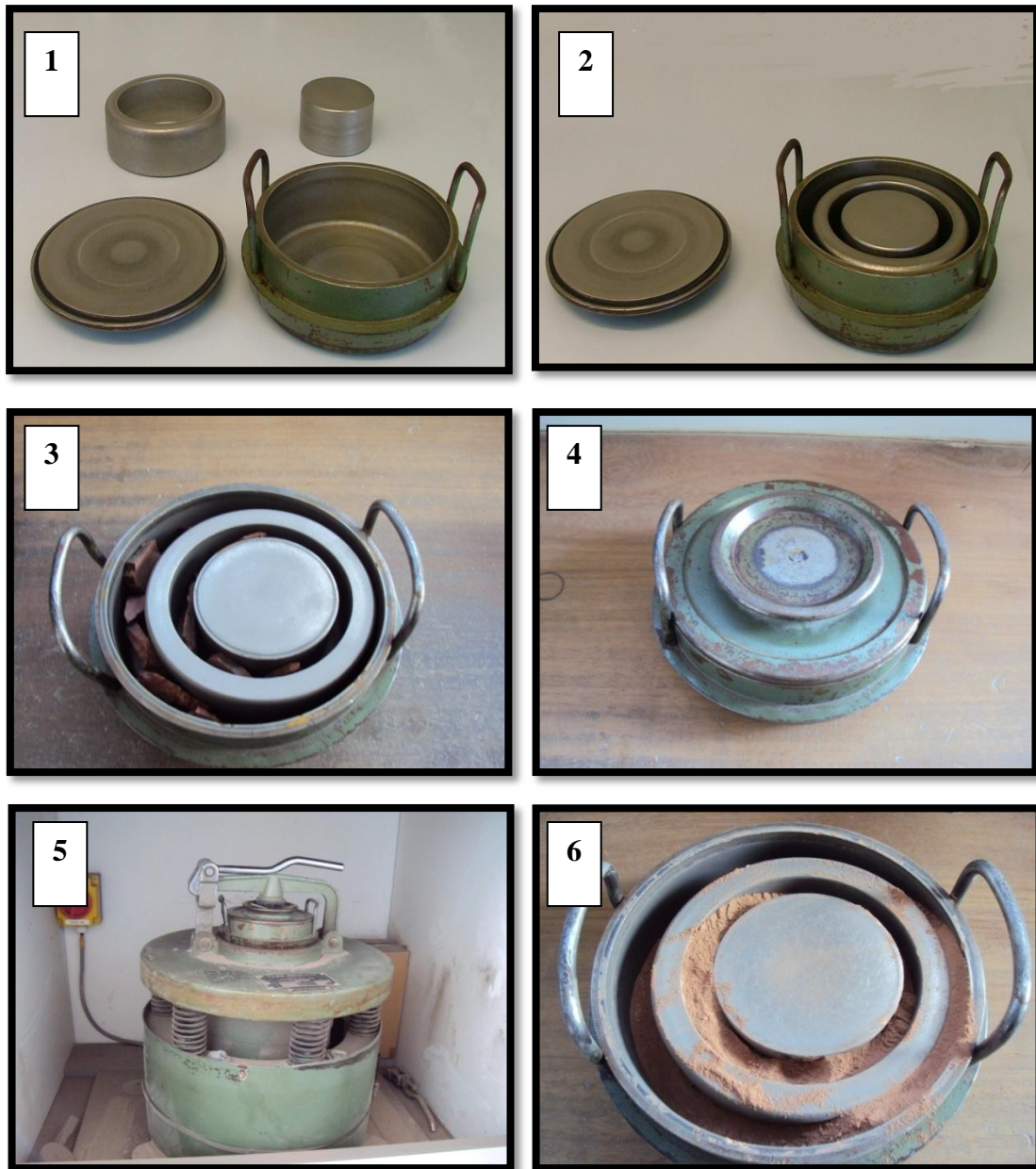
Figure 2.2: Mill used to prepare powdered samples at the University of Sheffield Department of Geography.
