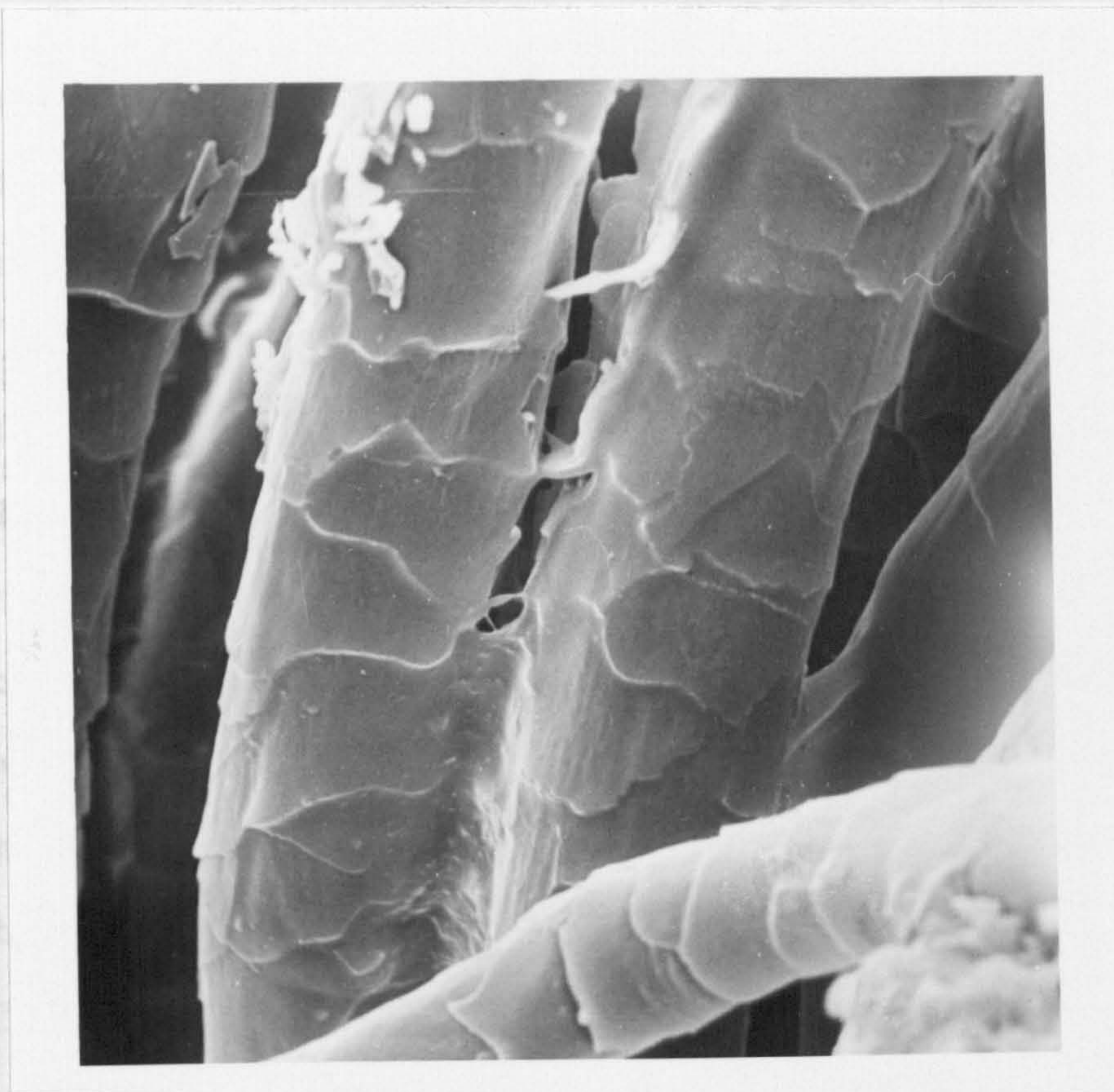
Fig. 64 - Woollen flannel - 2% Hercosett 125 applied by padding.
