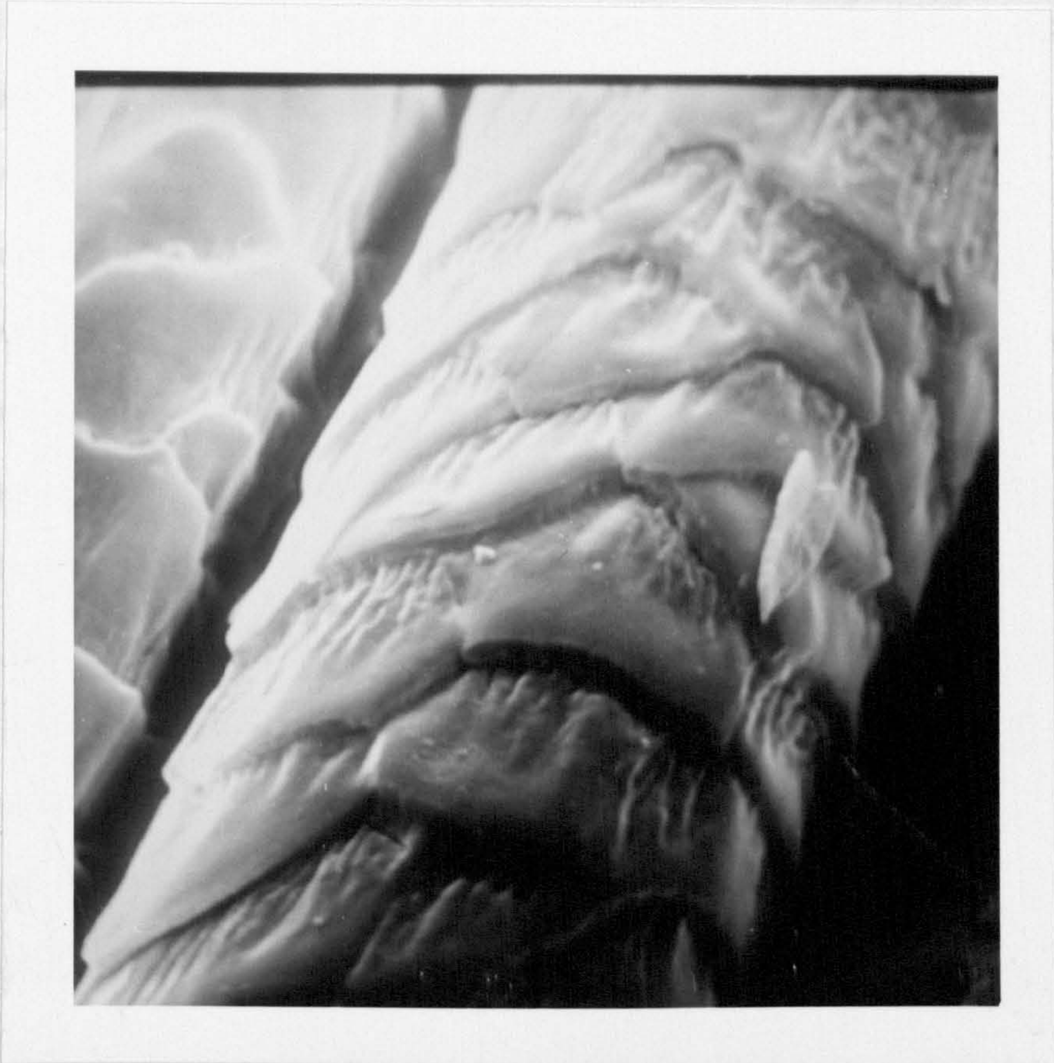
Fig. 102 - Wool fibre treated with ethylene glycol at 150°C for 60 s (2300X).
