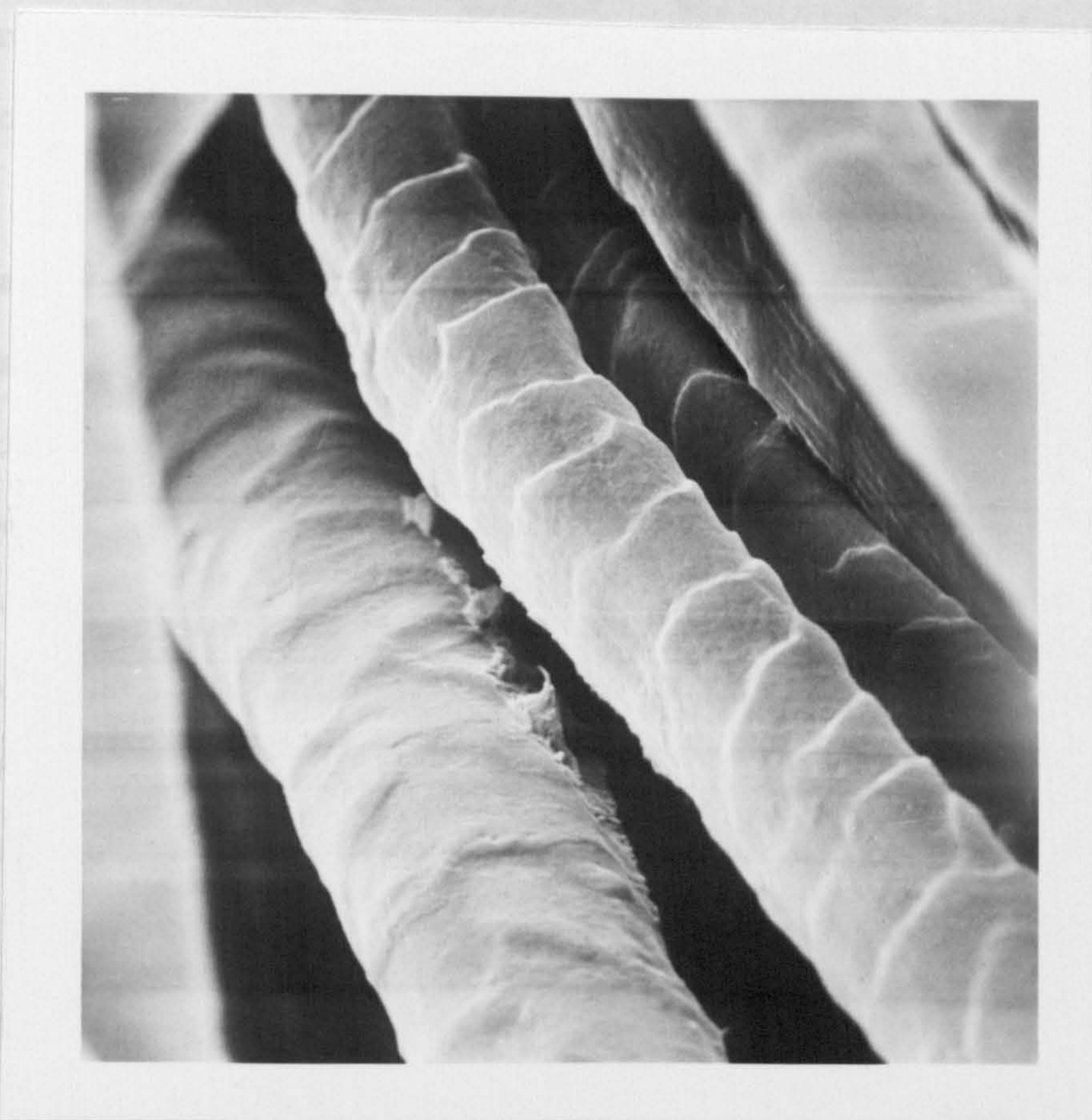
Fig. 65 - Woollen flannel - 2% Hercoestt 125 applied by exhaustion.
