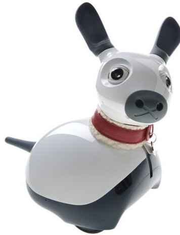
Fig. 4.2 The biomimetic MiRo robot is differentially driven and has a number of sensing options, though for this experiment only the sonar sensor, located in MiRo’s nose, is used for detecting walls. Whilst it is available both in physical form and simulated form, for ease of experimental setup, the simulated version of MiRo is used for testing our network model.
