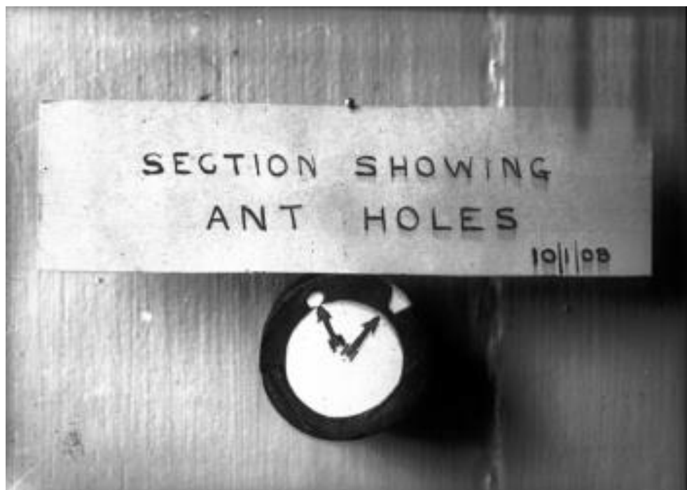
Figure 5.6: "Works photographic negative ant eaten cable, Calcutta". W. T. Glover & Co. Ltd, 1900 - 1910 [Science and Industry Museum Manchester Archives YA1972.36/MS0231/Neg 254]
