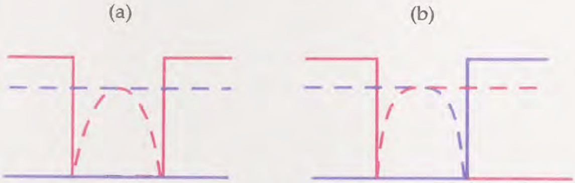
Figure 3.3 Spin dependent potentials and carrier densities (broken lines) for a magnetic trilayer sandwich, drawn for (a) ferromagnetic and (b) antiferromagnetic alignment. Red lines refer to the potentials experienced by (solid) and densities (broken) of spin-up electrons or spin-down holes, blue refers to spin-down electrons or spin-up holes.
