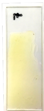
Figure 2.10: Prepared glass slide coated in a TAG film containing a mixture of 33.3 w/w% lard, 25 w/w% vegetable oil, 33.3 w/w% vegetable shortening and 8.3% linseed oil.
