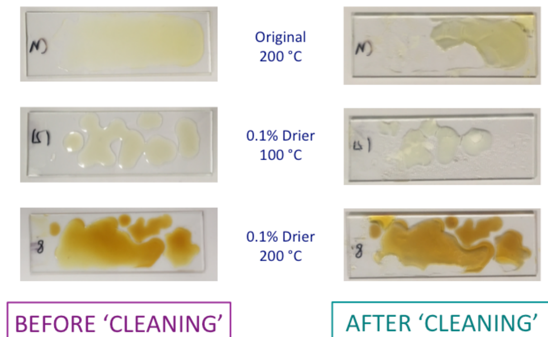
Figure 5.11: The TAG soils prepared under 3 different conditions: without drier and baked for 1 hour at 200 °C, with 0.1% cobalt 2-ethylhexanoate drier at 100 °C and 200 °C. The images on the left were taken after baking and before placing in the surfactant solution. The images on the right were taken after placing in a stirred surfactant solution (0.012% LO, 0.003% BC and 0.103% DG, with a pH was adjusted to 9) for 24 hours.
