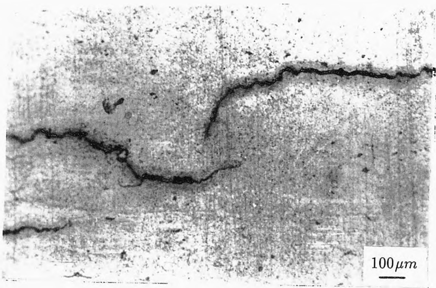
Fig.6.16 Typical example of crack coalescence achieved by the approach of two passing crack tips, f = 1 \text{ Hz} .
