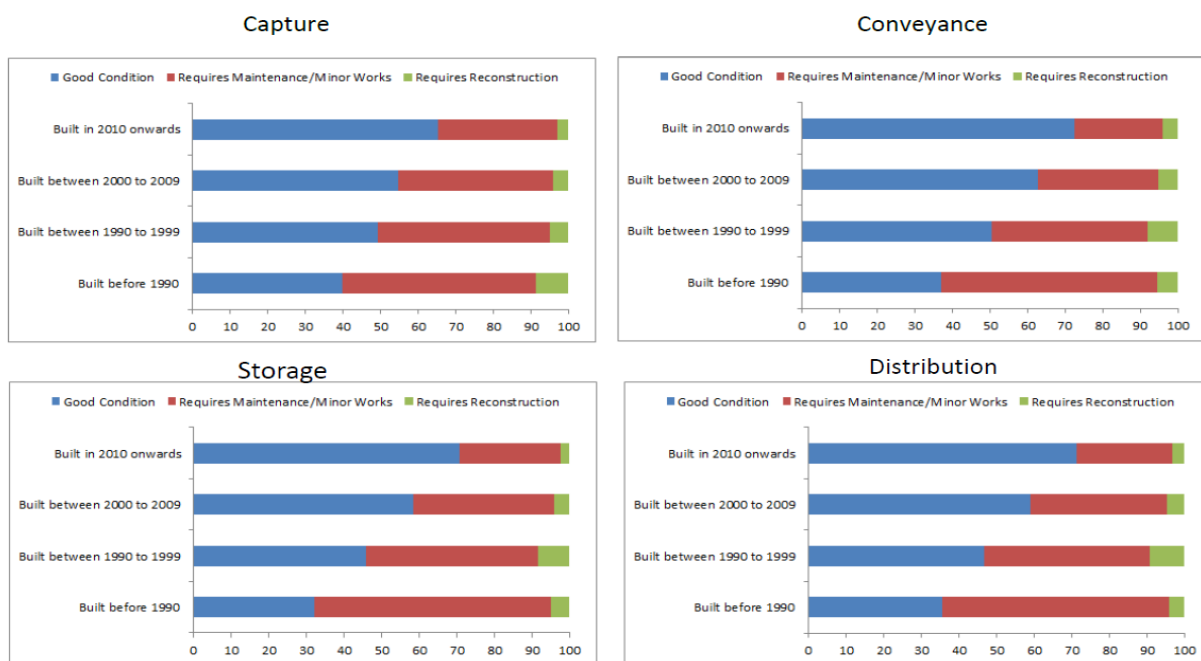
Figure 4-7 Physical Condition by Type of System and Quality Dimension, and Systems' Age Source: Own estimations based on SIASAR 2014-2015 Data.
