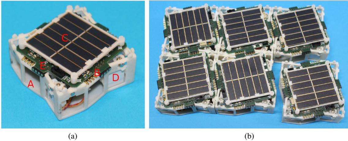
Figure 5.4 The evo-bot hardware. (a) A single evo-bot module, showing chassis (A), Connectors (B), solar cells (C), servo motors (D) and PCB (E). (b) Six evo-bot modules, five of which are connected.
