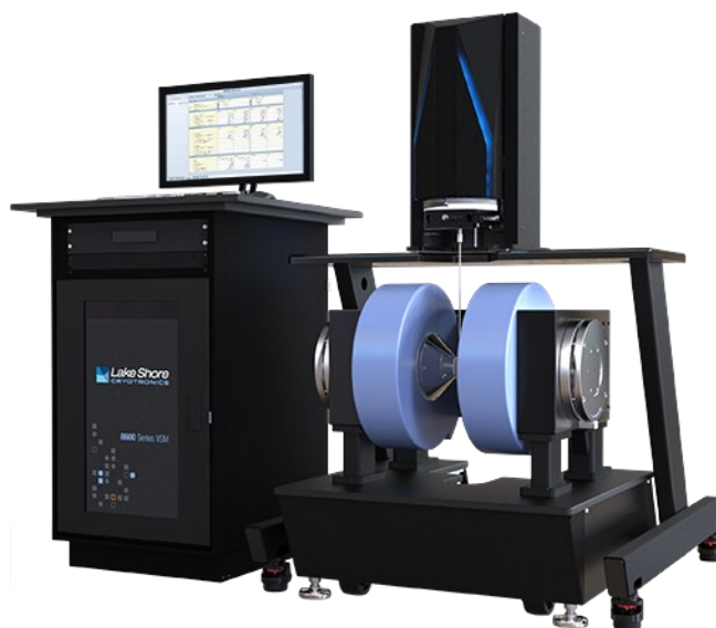
Figure 3.13: Picture of a lakeshore 8600 VSM [75].
