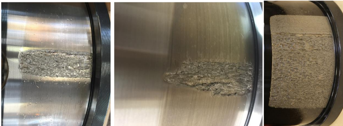
Figure 2-1: Examples of failed inner races of wind turbine gearbox bearings by flaking.
