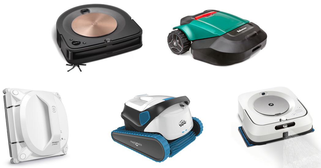
Figure 1.1: Examples of five commercially available coverage robots: iRobot Roomba s9 vacuum cleaner [89] (top left); Robomow RS635 lawn mower [160] (top right); Maytronics Dolphin S300i pool cleaner [132] (bottom left); Ecovacs winbot X window cleaner [56] (bottom center); and iRobot Braava m6 mop [88] (bottom right).
