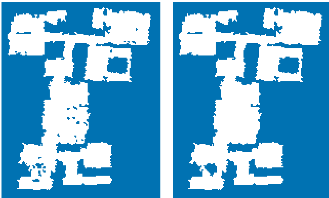
Figure 6.15: The raw binary occupancy grid map (left) contains many small obstacles and clustered obstacles. As a coverage robot can go around small obstacles without disrupting coverage and cannot go between the clustered obstacles, the small obstacles are removed and the clustered obstacles are connected in the simplified map (right).
