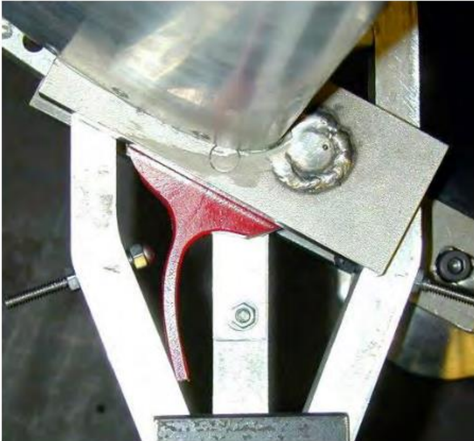
Figure 2.11 A photograph for a passive pitch mechanism based on a flexible stem [118].
