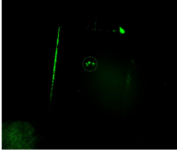
Figure 6.18: Background subtracted CTR image with analysis ROI centred over the emission region by eye. Circular ROI of 200 pixel diameter. ImageJ Raw Integrated Density function was used to sum the signal contained within the ROI.
