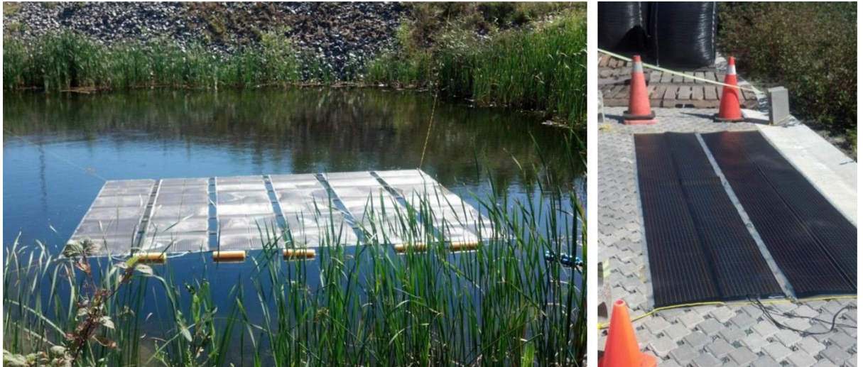
Figure 2-16: Floating PV panels (Trapani and Millar, 2014).
