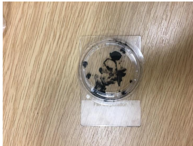
Figure 4.4 Dried soot particles after drying in a vacuum oven at 60°C for 24hours
