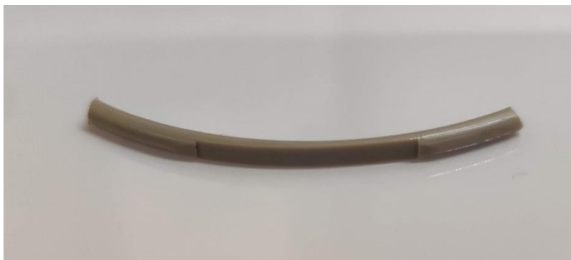
Figure 9.13 Worn PEEK after test
