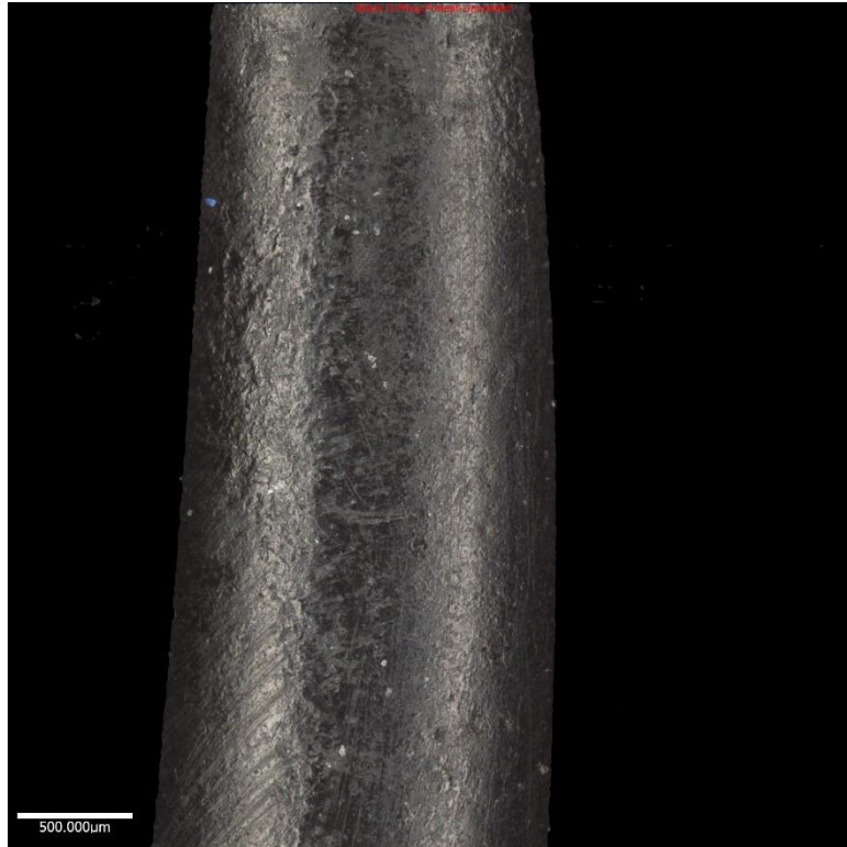
Figure 9.20 Worn NBR ring after test
