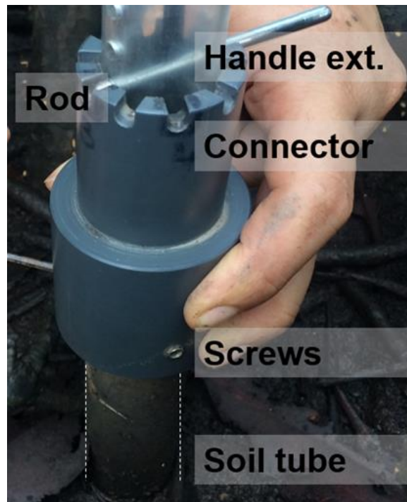
Figure 2-5 EnRoot's indexing handle and soil tube connector allow images to be taken at precise depths and radial directions within the soil tube. The screws hold the connector in place.
