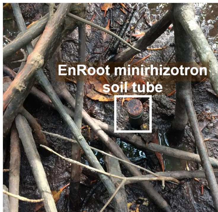
Figure 2-8 An EnRoot soil tube installed between stilt roots of mangrove trees in Vietnam.
