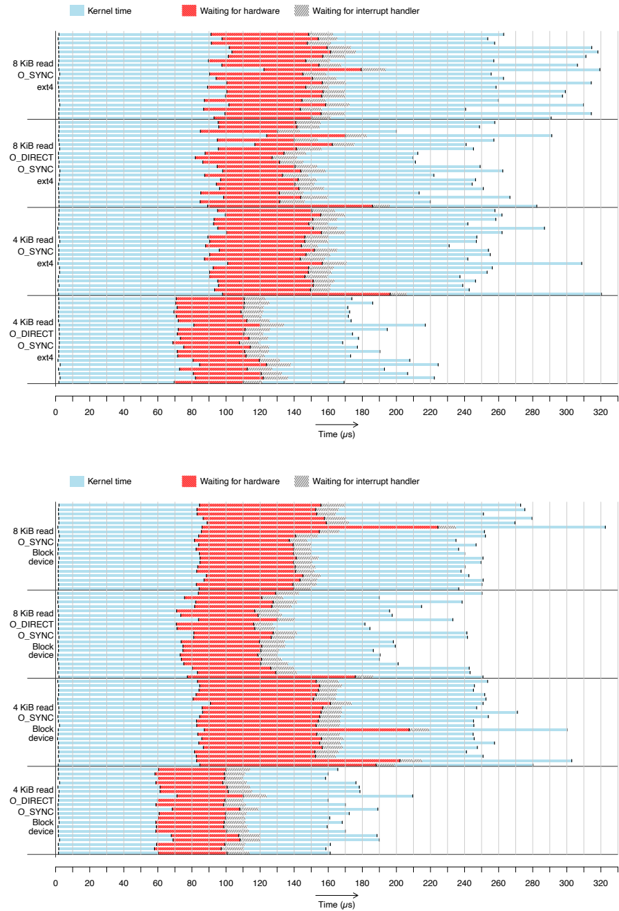
Figure 3.26: Profiling results for 20 runs each of 4 KiB and 8 KiB reads, with and without direct I/O, from ext4 (top) and NVMe block device (bottom)
