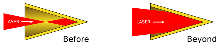
Figure 4.1: Focusing the laser before the cone tip and beyond the cone tip. In this chapter the convention is used that a negative defocus position is before the cone tip and a positive defocus position is beyond the cone tip.
