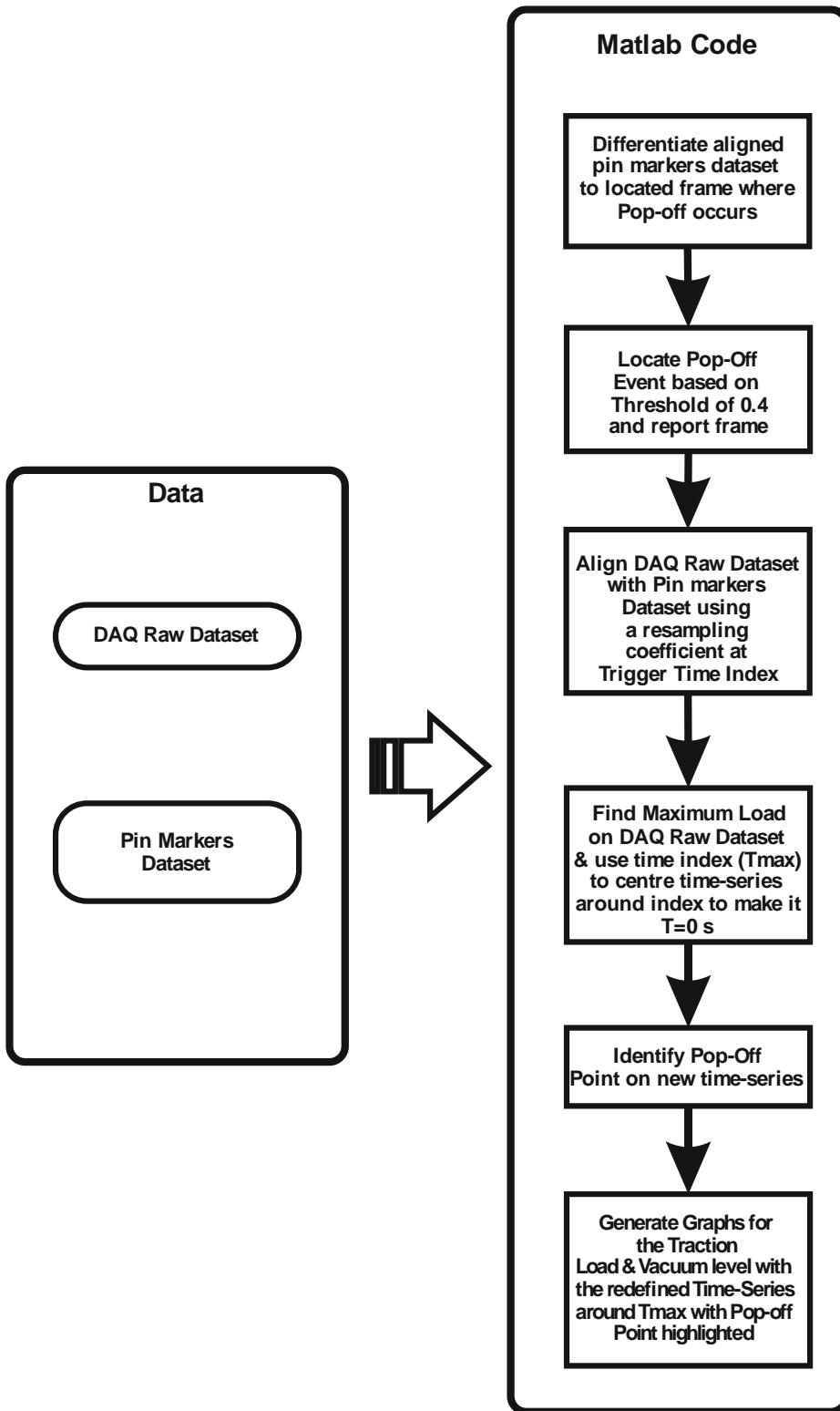
Figure 4-27: Data Processing flowchart for the acquired pin markers and DAQ data sets
