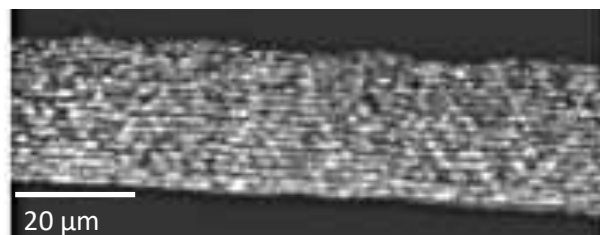
Figure 1.6: Optical micrograph show a multi-layered oxide structure formed after aqueous corrosion tests at 360°C for 784 days Zircaloy-4 [63].
