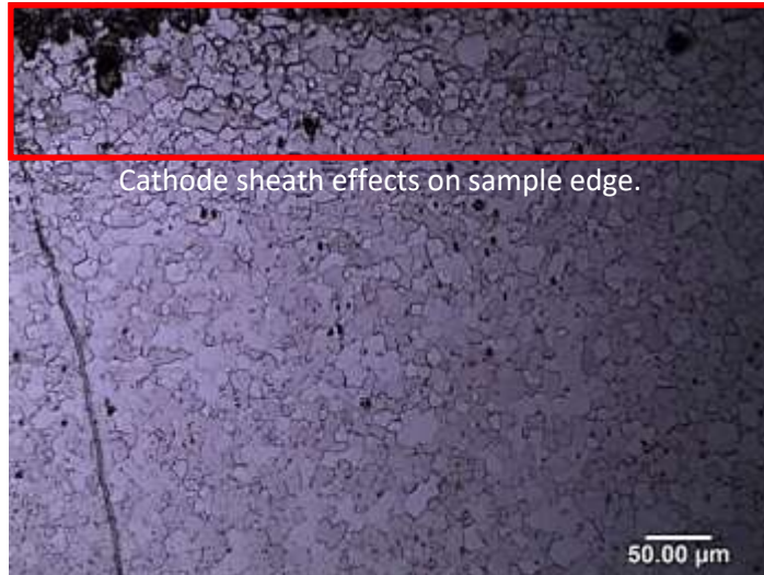
Figure 3.8: Optical micrograph of the 4 hr TPN-treated Zr showing more pronounced Zr microstructure towards the edge of the TPN-treated surface due to cathode sheath edge effects.
