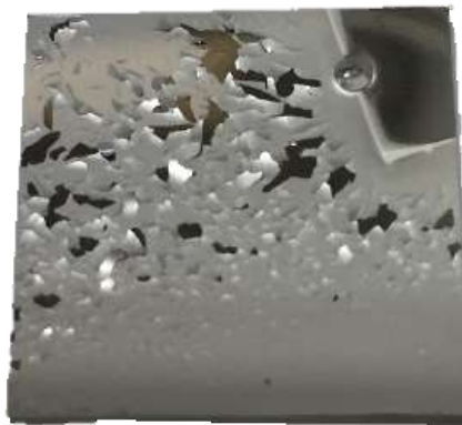
Figure 5.2: Camera image showing spallation of the Zr-Mg coating on zirconium substrate when the sample was taken out of the deposition chamber following 5 min cooling time.
