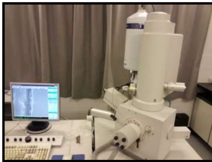
Figure 2.9: Philips SEM XL30 was used to analyse the surface morphology.
