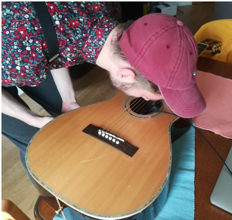
Fig. 15. Positioning the microphone inside the guitar.
