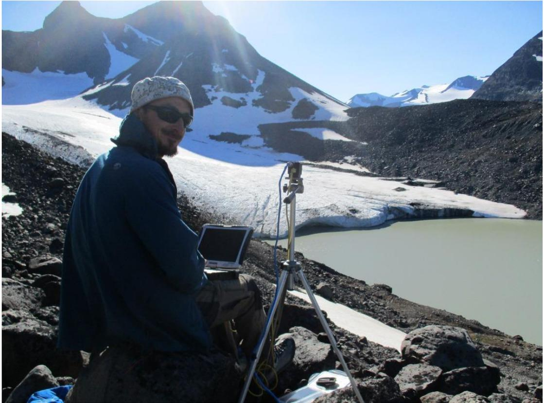
Figure 4.13 Conducting a preliminary thermal infrared survey from ‘Owl’s nest’ position on the eastern lateral moraine with FLIR A65 thermal camera (see 0Figure 4.8 for location). Photo: Tom Sloan (24/7/2017).
