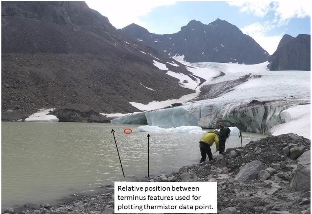
Figure 4.12 Timelapse image (GoPro Hero4) taken from the terminus survey position (Tr) showing prominent landforms used for triangulation and spatial plotting of temperature data. Note the large ice berg from the 26<sup>th</sup> July calving event, which is sitting directly in front of the section of terminus that it calved from (see Figure 4.18).
