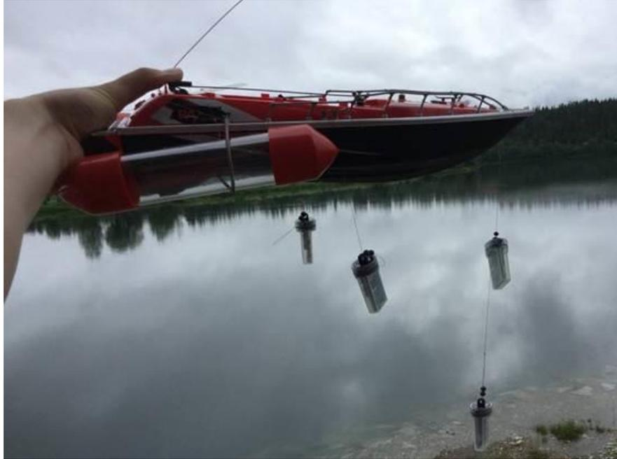
Figure 4.10 The remote controlled boat with HOBO thermistors that was used for surface temperature surveys. Note the weighting to maintain thermistor position. A further HOBO thermistor was installed on the boat deck to monitor air temperature during the survey. The boat is 40 cm long.
