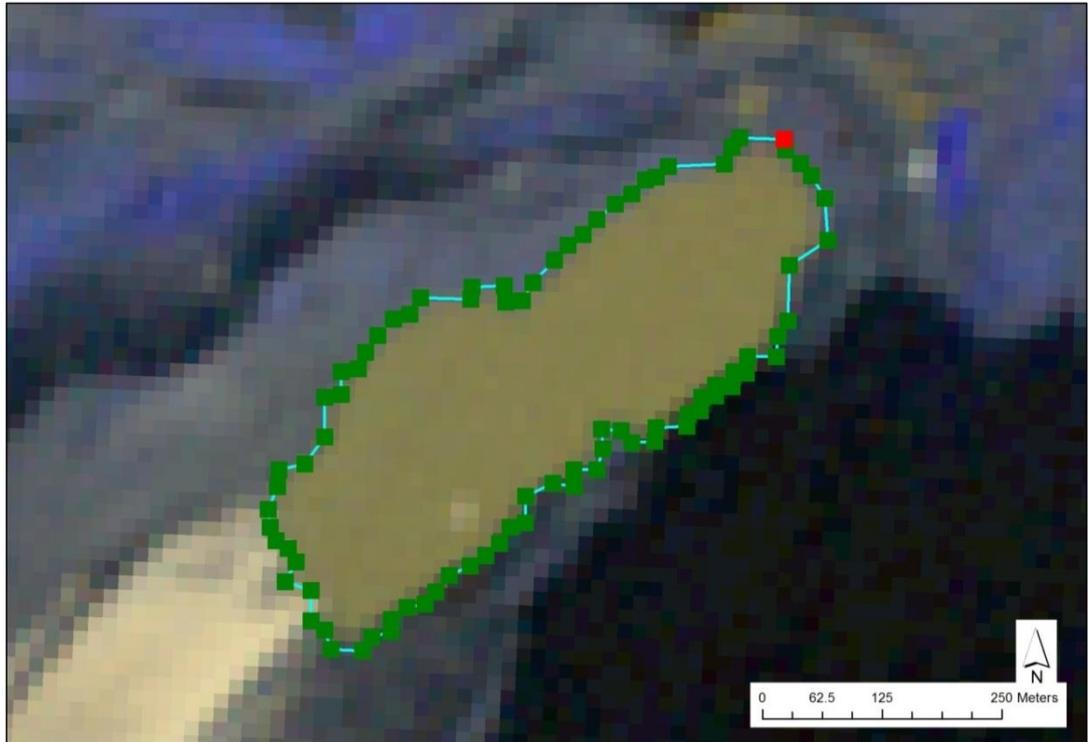
Figure 2.2.2 Satellite image from ASTER of Kaskasapakte glaciaren proglacial lake (PGL<sub>ID</sub>24, 132,172 m<sup>2</sup>), displayed as a composite of green, red and near infrared (bands 1, 2, 3N; all 15 m resolution) showing vertices for proglacial lake manual mapping.
