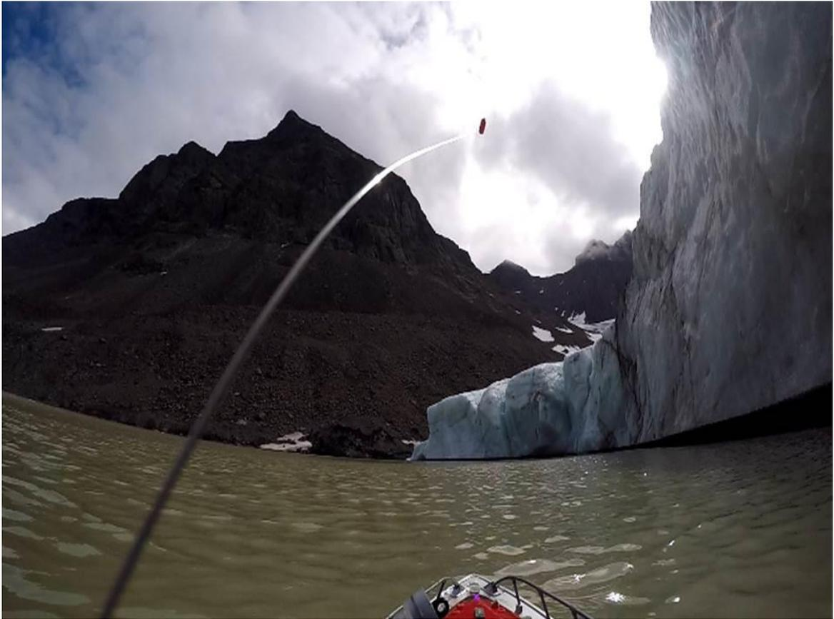
Figure 4.20 Image from GoPro Hero4 camera from remote controlled boat survey of Kaskapakte glacier, Arctic Sweden (A.Dye, 4/8/2017). Note the thermally eroded notch shadow extending along the glacier terminus at the water to ice contact point. The height of the subaerial ice cliff is estimated to be ~5 m.
