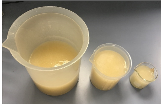
Figure 2-5: Demineralising gel (neither thick nor runny).
