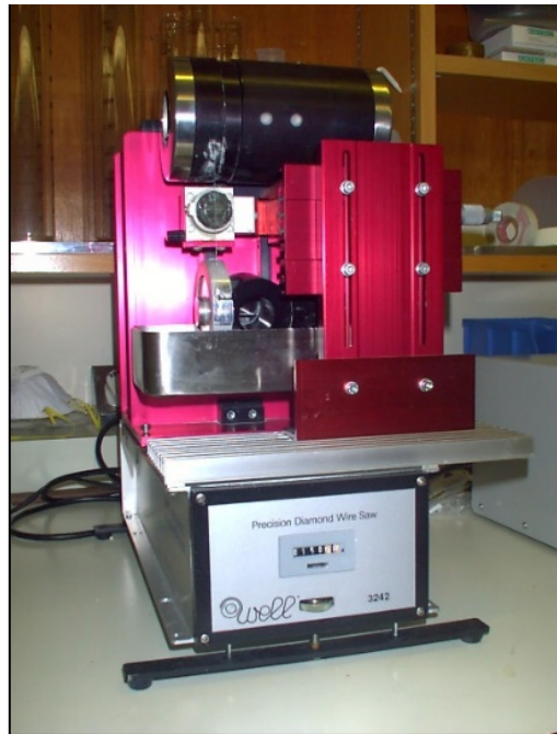
Figure 2-3: Teeth cutting using diamond wire saw machine (Well® Walter EBNER, CH-2400 Le Loche). Notice the final size and the thickness of the enamel slab.
