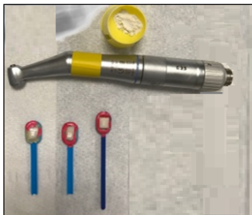
Figure 2-18: Slow-speed handpiece, soft rubber cup and extra-fine pumice grit were used to polish the enamel slabs.
