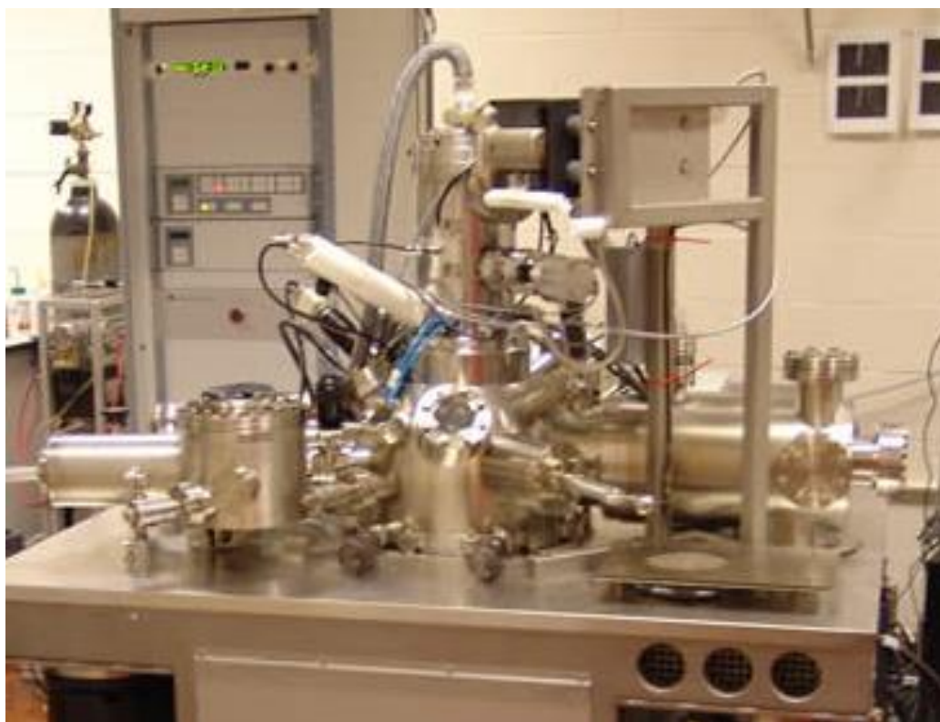
Fig 2.6 The 4-probe Scanning Probe Microscope used for the electrical characterisation of the M13 gold nanowire.
