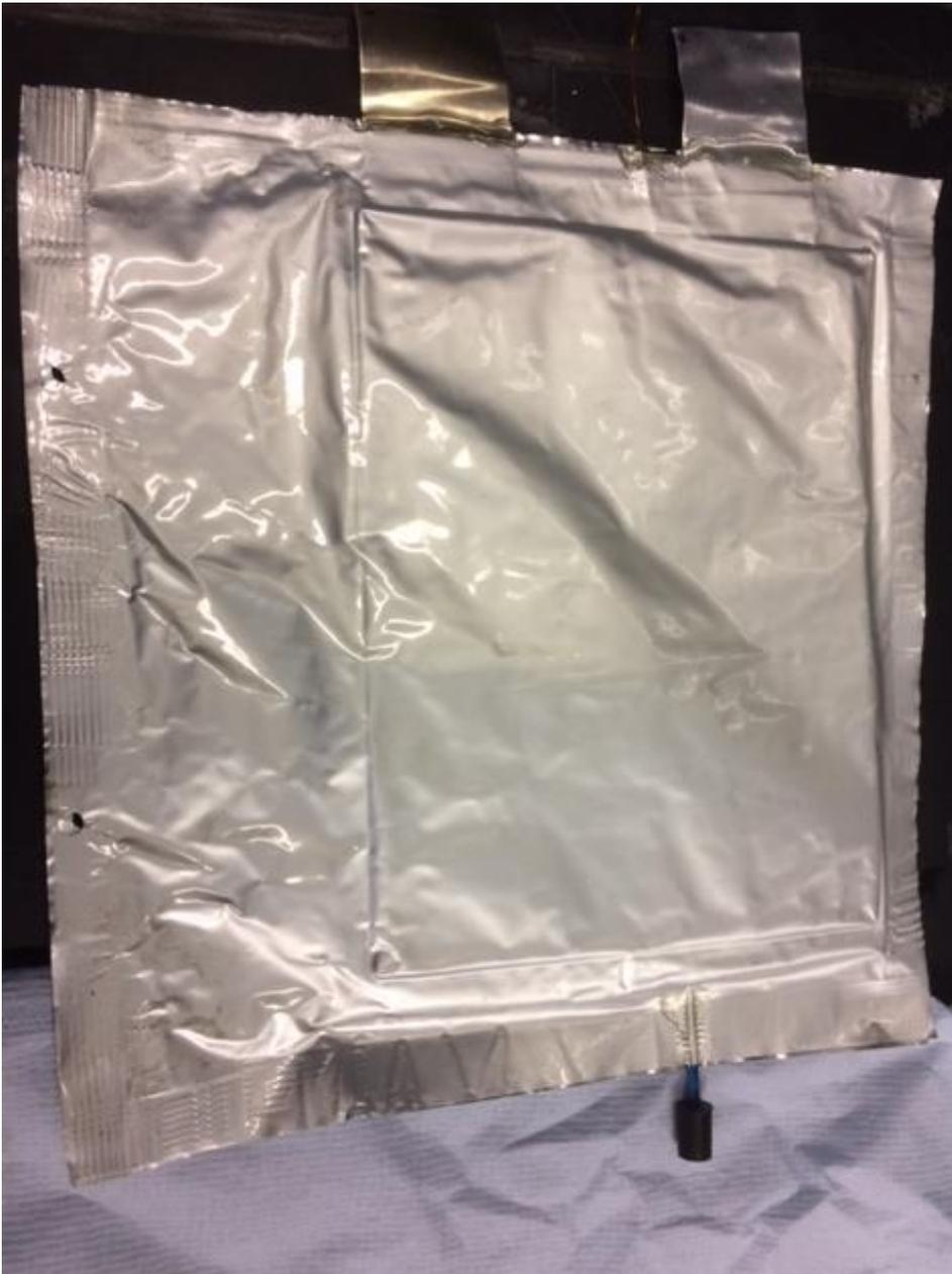
**Figure 5.13 Completed large capacity Lithium ion pouch cell with embedded ZBLAN fibre optic and thermocouple inserted through opposite edges of pouch**
