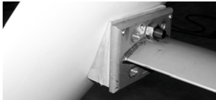
Figure 3.3: Armstrong and Tullis’ blade support arm joint, as used to adjust fixing angle [78].
