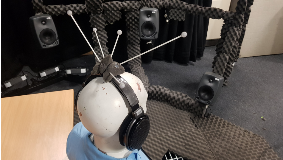
Figure 7.1: 5-point array of reflective markers secured to sennheiser HD650 headphones for the purpose of head-tracking
