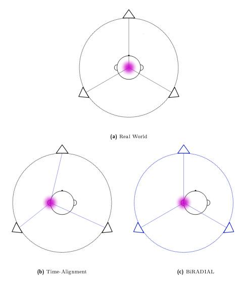
Figure 5.2: Examples of a) real world, b) Time-Alignment and c) BiRADIAL Ambisonic rendering and the positioning and optimization the sweet spot for binaural reproduction. Note that the examples in Fig. 5.2b and 5.2c are only being shown for the left ear and would ordinarily also be performed separately for the right ear. The approximate location of the sweet spot is in each case highlighted in purple.
