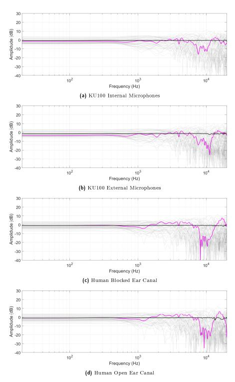
Figure 7.3: Spectral plots of the KU100 and human HRTFs measured in MARC with internal/external microphones and a blocked/open ear canal respectively. Diffuse-field equalised HRTFs are shown in grey. The HRTF of angle ( $\varphi=0^{\circ},\vartheta=0^{\circ}$ ) is highlighted in purple. The diffuse-field response of the diffuse-field equalised HRTFs is shown in black.
