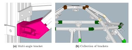
Figure 6.10: Construction of the frame using 3D printed angle brackets to sit perpendicular the loudspeaker angles.
