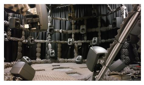
Figure 4.14: The 50 point spherical loudspeaker array housed in AudioLab, Genesis 6, University of York. The array has been treated with acoustic foam in an attempt to reduce reflections.
