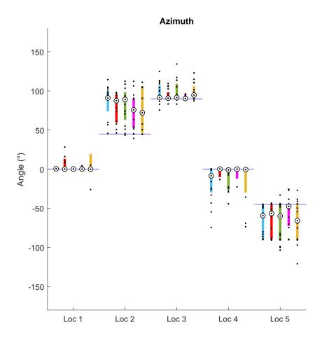
Figure 7.12: Azimuth localisation results. Source locations are grouped upon the y-axis. The correct location is depicted by a horizontal blue line. Median values are presented as a black dot within a solid white circle. Each of the 5 renderers are identified by colour (and lateral position).
