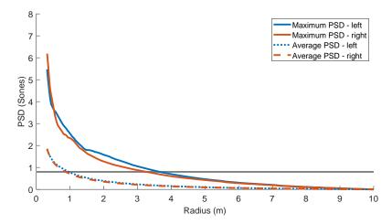
Figure 6.4: Average and maximum PSD between radially-spaced HRTFs and the 10m reference for an incident angle of  $(\varphi = 0^{\circ}, \vartheta = 0^{\circ})$ . The horizontal line represents the JND of 0.8 Sones.
