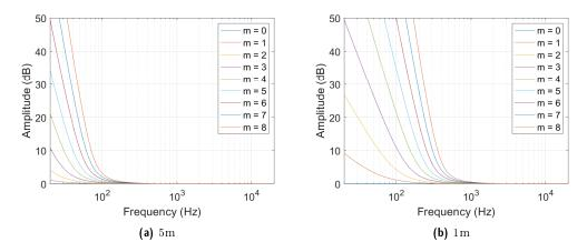
Figure 4.7: Bass boosting amplitude response of the near-field effect filter for degree,  $m=0,1,\ldots 8$ , for a source simulated at a) 5m b) 1m
