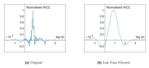
Figure 2.6: Example of the InterAural Cross-Correlation (IACC) an HRTF azimuth =  $90^{\circ}$ , elevation =  $0^{\circ}$  with and without low pass filtering. Note the single clean and easily identifiable peak in the resulting waveform.
