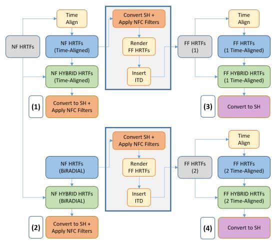
Figure 6.36: An outline of the 4 methods (1-4) suggested to produce far-field Ambisonic decoders (weighted HRTFs encoded into spherical harmonic format) from a set of near-field measurements. The 3-step process highlighted by the light blue background is the synthesis of far-field HRTFs.
