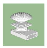
(c) -90° elevation loudspeaker in 3D printed casing with protective grill
