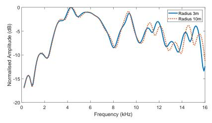
Figure 6.7: Left channel of HRTF for  $\vartheta=\pm45^\circ$ ,  $\varphi=35.3^\circ$ , simulated at 3m and 10m, normalised such the the maximum value of each HRTF equals 0dB. Note the misalignment of high frequency notches resulting in a high maximum PSD.
