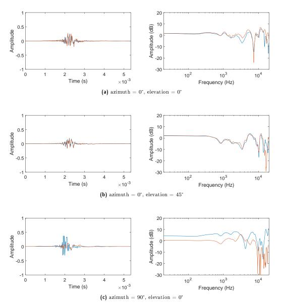
Figure 2.15: Time and Frequency domain plots of 3 binaurally rendered stereo HRTFs reproduced with  $3^{\rm rd}$  order Ambisonics over a 1.2m radius virtual array with KU100 HRTFs measured as part of the SADIIE database, see Section 3.3. Blue: Left ear, Red: Right ear. Amplitude is shown on the y-axis (in dB for frequency domain plots).
