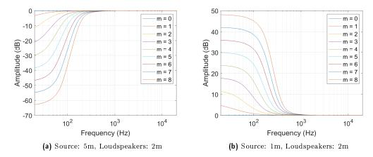
Figure 4.8: Shelf filtering amplitude response of the combined near-field effect and compensation filters for degree,  $m=0,1,\ldots 8$ , for a loudspeaker radius of 2m and a source simulated at a) 5m b) 1m
