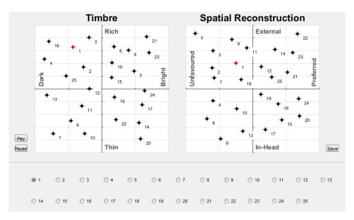
Figure 3.10: The graphical interface used by participants to rate audio stimuli. Selection of stimuli was made using the radio buttons at the bottom of the interface. A corresponding marker would be highlighted on each graph and participants were required to click and drag the markers using a computer mouse to where they felt was appropriate.
