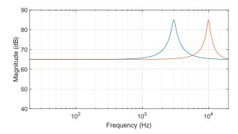
Figure 5.19: Frequency response plots of 3 kHz (blue) and 10 kHz (red) +20 dB peak filters with each bandwidth equal to the ERB of those frequencies.
