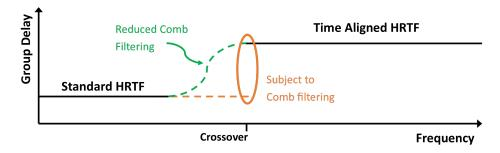
Figure 5.6: Implementation of a gradual group delay filter to smooth the transition between the standard and Time-Aligned HRTFs.
