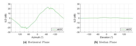
Figure 2.8: Example of the ILDs on the Horizontal (left) and Median (right) plane for the KU100 dummy head and a source at 1.2m radius (data from the SADIIE database, see Section 3.3). A positive value indicates that the sound is louder in the right ear compared to the left.
