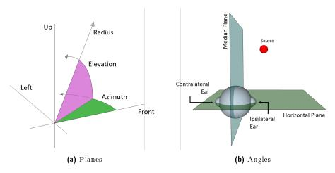
Figure 2.1: Basic coordinate system where azimuth is measured anticlockwise about the horizontal plane and elevation is measured from the horizontal place (upward positive). Radius is measured outward from the origin. Ipsilateral and contralateral ears are defined by the placement of a source either side of the median plane.
