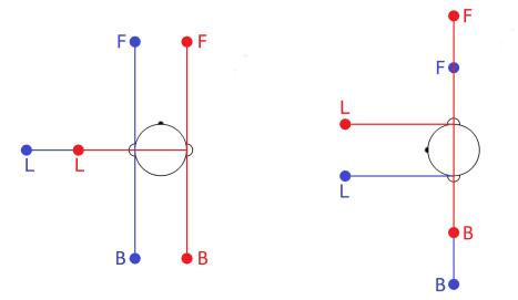
Figure 5.11: The rendered locations of three sources (ideally positioned to the Front (F), Left (L) and Back (B) of a listener) for left (blue) and right (red) Bi-RADIAL loudspeaker arrays. Locations are shown for two listener orientations. Note the corresponding  $90^{\circ}$  counter-rotation of the soundfield.
