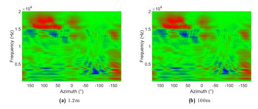
Figure 6.44: Comparison of the PSDM (left channel only) of BiRADIAL intermediate generation and re-synthesis of far-field HRTFs 2702 points at 1.2 and 100m. Comparisons are made with respect to SADIIE HRTFs.
