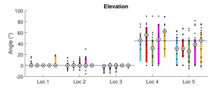
Figure 7.13: Elevation localisation results. Source locations are grouped upon the y-axis. The correct location is depicted by a horizontal blue line. Median values are presented as a black dot within a solid white circle. Each of the 5 renderers are identified by colour (and lateral position).
