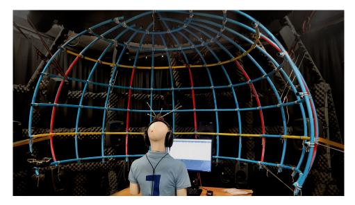
Figure 7.8: The colour coded reference grid that surrounded the participant. Red and yellow highlights define 45° increments about the azimuth and elevation.
