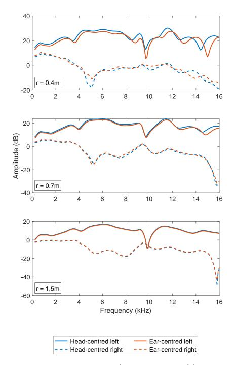
Figure 6.8: Laterally spaced HRTFs simulated from an incident angle of  $\vartheta=90^\circ$ ,  $\varphi=0^\circ$  at the radial distances of: 0.4m (top), 0.7m (middle) and 1.5m (bottom). The settling of spectral features with an increase in distance can be seen.
