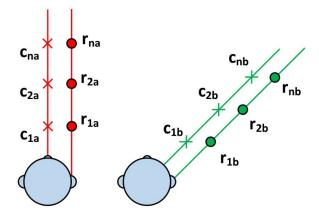
Figure 6.3: Laterally spaced HRTFs: at each angle (a, b, ...) a series of head centred HRTFs  $c_1, c_2, \ldots, c_n$  are compared to a series of ear centred HRTFs  $(r_1, c_2, \ldots, c_n)$  such that the left channel of the head centred HRTF is compared to the left channel or the left ear centred HRTF and vice versa for the right. The diagram shows the comparison for the right ear only
