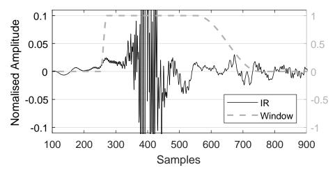
Figure 3.5: Windowing of HRTFs to 500 samples by means of a 20 sample half Hanning window and 130 sample pad before each peak and a 150 sample pad and 200 sample half Hanning window after. Note that the plot has zoomed in on the IR to illustrate the region of windowing.
