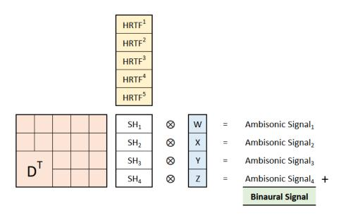
(b) Spherical harmonic domain approach.  $D^T$  is the transposed decoding matrix; [W, X, Y, Z] is the Ambisonic input file. SH are the spherical harmonic format HRTFs.
