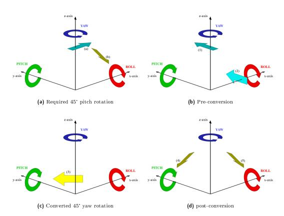
Figure 4.18: Implementation of a pitch rotation (a to b) by means of pre- and post-  $90^{\circ}$  conversion rotations and a variable yaw rotation. First a  $90^{\circ}$  yaw (1) is followed by a  $90^{\circ}$  pitch (2). The variable rotation is then performed as a yaw (3). The conversion is then inverted by a  $-90^{\circ}$  pitch (4) and a  $-90^{\circ}$  yaw (5).
