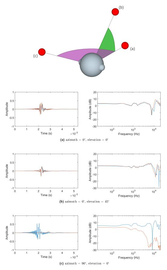
Figure 2.13: Time and Frequency domain plots of 3 stereo HRTFs measured at 1.2m radius as part of the SADHE database of the KU100 dummy head, see Section 3.3. Blue: Left ear, Red: Right ear. Amplitude is shown on the y-axis (in dB for frequency domain plots).
