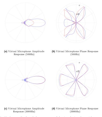
Figure 6.35: Absolute amplitude and phase responses of the virtual microphone pick up patterns for a a&b) 500Hz and c&d) 3000Hz) panned to 0° and simulated at a distance of 100m to be rendered over a 0.5m and 1m radii loudspeaker array using NFC filters. Blue: the response of the  $100 \rightarrow 1m$  NFC filter. Red: the response of the  $100 \rightarrow 0.5m$  NFC filter.
