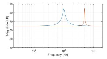
Figure 5.22: Frequency response plots of 1 kHz (blue) and 5 kHz (red) +20 dB peak filters with 100 Hz -3 dB bandwidths.
