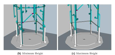
Figure 6.14: Adjustable height operation of MARC via 4 linear actuators mounted between the floor and an internal frame (highlighted blue). Attachment of the internal frame to the fixed basket by pairs of roller wheels is shown in Fig. 6.14a.
