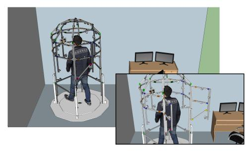
Figure 6.9: Original Sketch Up $^{23}$  concept design of MARC, a walk-in near-field HRTF measurement rig.
