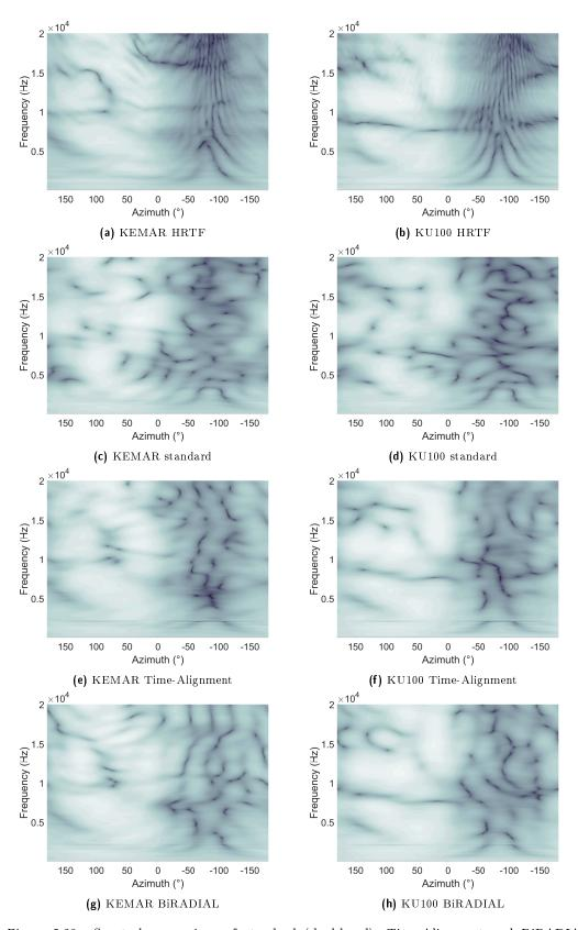
Figure 5.28: Spectral comparison of standard (dual-band), Time-Alignment and BiRADIAL binaural  $5^{\rm th}$  order Ambisonic rendering methods using 1.2m KU100 and KEMAR HRTFs from the SADIIE Database. Data is taken in 1° increments about the horizontal axis. Amplitude is shown by colour. Black: -60dB, White: +20dB.
