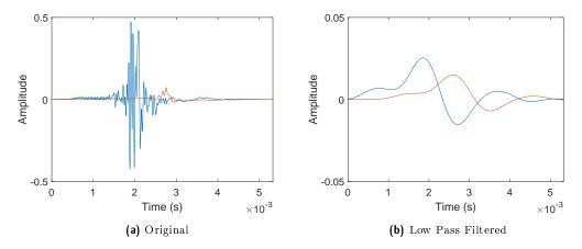
Figure 2.5: Example of an HRTF azimuth = 90°, elevation = 0° before and after low pass filtering. Note how the high frequency noise has been removed a more obvious time delay between the waveforms is visible. Blue: Left Signal. Orange: Right Signal.
