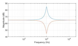
Figure 5.21: Frequency response plots of 1 kHz +20 dB peak (blue) and -20 dB notch (red) filters.
