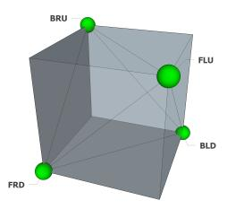
Figure 4.2: Example of a tetrahedral microphone configuration with microphone angles based on the vertices of a cube labelled as Front, Back, Left, Right, Up and Down.
