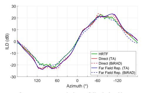
$Figure \ 6.38: \ Comparing \ ILD \ estimations \ for \ direct \ NFC \ filtered \ spherical \ harmonic \ rendering \ against intermediate \ generation \ and \ re-synthesis \ of \ far-field \ HRTFs$
