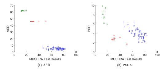
Figure 5.23: Comparison of the Absolute and Perceptual Spectral Difference calculations plotted against real MUSHRA listening test data. Data includes true reference and low pass anchors. Note that whilst the ASD is representative of an average difference between stimuli in dB, PSDM is better described as a perceptually weighted average difference between stimuli in Sones. Black: Hidden reference, Red: Mid-Anchor, Green: Low Anchor, Blue: Test stimuli.
