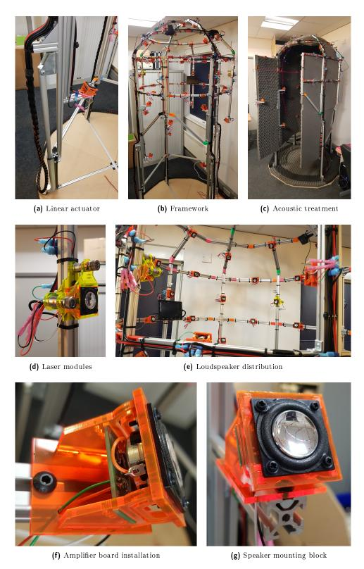
Figure 6.17: Finished prototype of MARC showing some of the key features.
