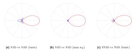
Figure 4.6: Virtual microphone pickup patterns of  $3^{\rm rd}$  order projection decoders. a) and b) show correctly normalised basic and max- $r_E$  decoders respectively. c) shows the result if SN3D normalised data is input to an N3D normalised basic decoder. Note that in the case of both b) and c) the rear lobing is reduced at the expense of a slight widening of the frontal lobe.
