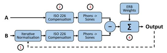
Figure 5.14: Flowchart of the PSDM showing the comparison of input spectra A and B
