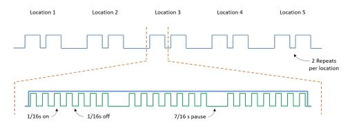
Figure 7.9: Pulse train sequence for testing the localisation performance of each renderer
