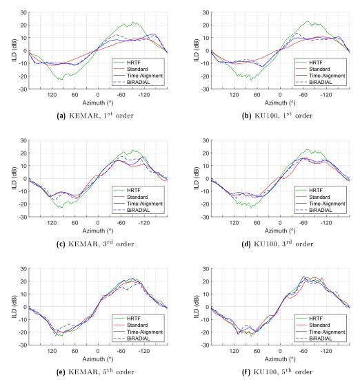
Figure 5.27: ILD comparison of standard, Time-Alignment and BiRADIAL binaural Ambisonic rendering methods using 1.2m KU100 and KEMAR HRTFs from the SADIIE Database. Data is taken in 1° increments about the horizontal axis. ILD is calculated from band-limited signals above 1500Hz.
