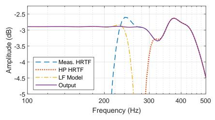
Figure 3.3: The 275Hz crossover of a measured HRTF and individually generated low frequency model.
