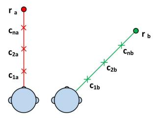
Figure 6.2: Radially-spaced HRTFs: at each angle (a, b, ...) a series of HRTFs (c<sub>1, 2, ... n</sub>) are each compared to a reference of the same angle, but a 10m radius (r).
