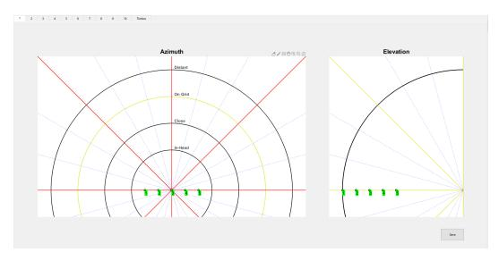
Figure 7.7: Matlab GUI for inputting perceived location of sources. Subject is asked to input azimuthal and radial position on the left, and elevation on the right. Radial positions are labelled: 'In-Head', 'Close', 'On Grid' and 'Distant'.
