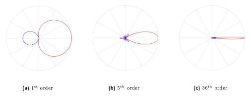
Figure 4.10: 1<sup>st</sup> (left), 5<sup>th</sup> (middle) and 36<sup>th</sup> (right) order Ambisonic representations of a point source. Positive values are shown in red. Negative (out of phase) values are shown in Blue.
