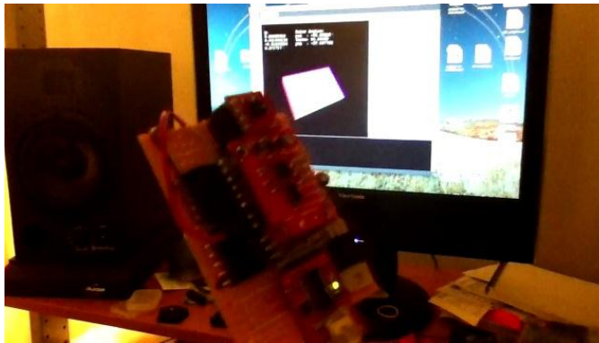
Centeno's head tracker device based on Arduino, to be mounted upon a headphone. Derived from http://vimeo.com/22727528 .
