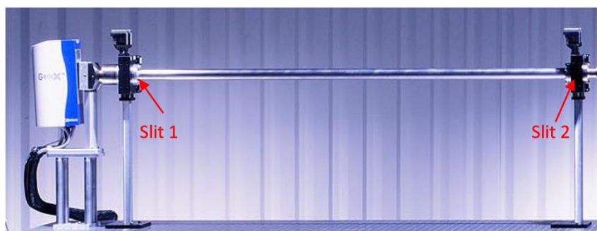
Figure 4-5 X-ray source of Xeuss system and the two slits in the pencil tube.
