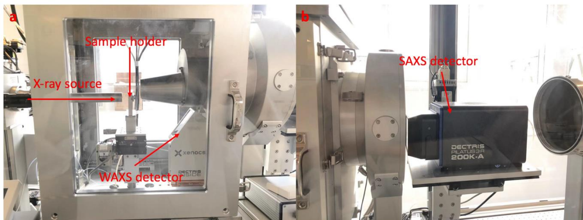
Figure 4-6 The detectors in Xeuss system.
