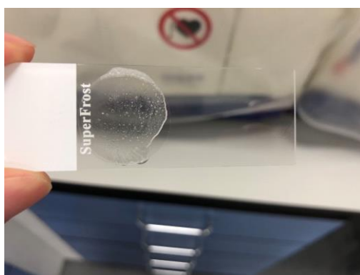
Figure 4-4 The sample for hot-stage microscopy. Air bubbles were appeared in the sample.
