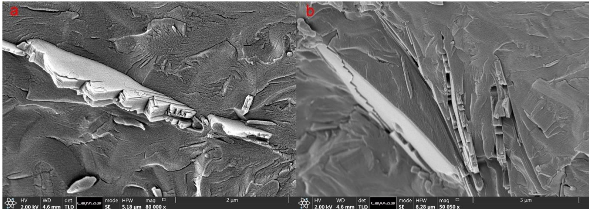
Figure 6-18 The cryo-SEM images of the sample prepared with PSFA. Lamellar crystals dispersed in amorphous non-ionic surfactant. The sharp interfacial area was observed in a. The scale bars are: 2 \mu m (a) and 3 \mu m (b).
