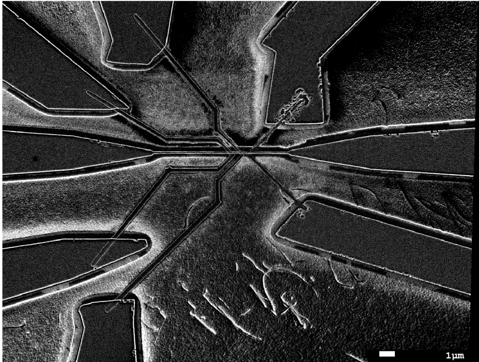
Figure 4.5: Subtraction images after their contrast has been rescaled. This sample is an array of 100 nm wide Cu, Pt and Permalloy wires deposited on \text{SiO}_2 . The deposited wires should also be 100 nm thick. The voltages used were 2 and 3 keV.
