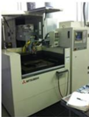
Figure 6-21: Contour measurement set up: (a) Wire EDM machine, (b) Surface roughness measurements.
