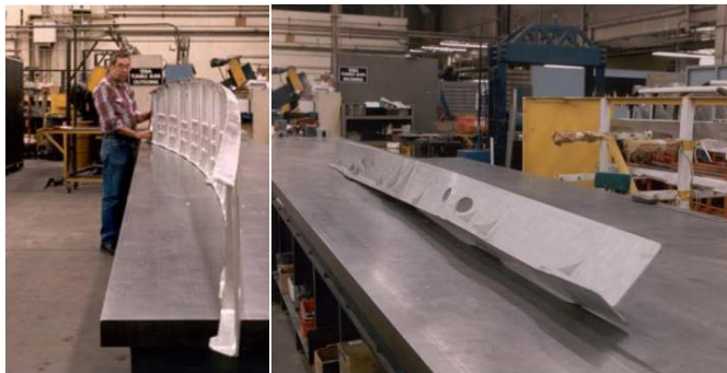
Figure 1-7: Machining generated distortion on aerospace components [21].
