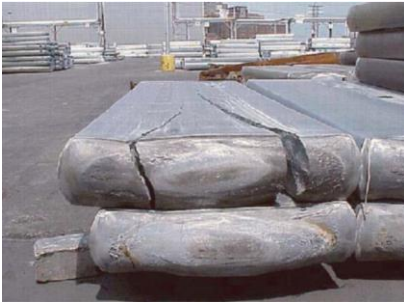
Figure 2-4: (a) Cracking in a cast aluminium ingot due to excessive residual stresses [15], (b) Thin wall-floor aluminium component [45].
