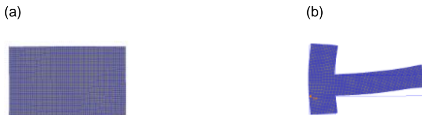
Figure 4-9: One-step machining distortion simulation: (a) Pre heat treatment geometry, (b) Final part geometry with distortion.
