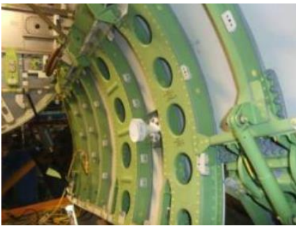
Figure 1-6: Conversion of an aluminium structure; (a) Assembled structure, (b) Monolithic structure.
