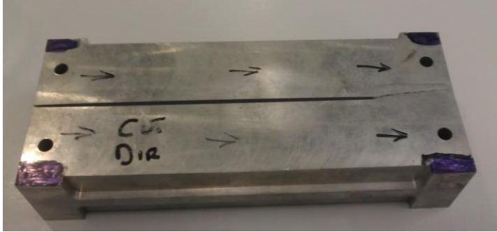
Figure 7-12: Crack across coupon caused due to excessive residual stresses generated during the quenching process.
