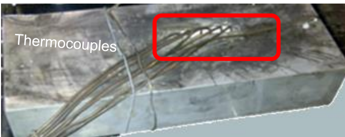
Figure 6-15: Experimental set up for: (a) Quench tank (b) Top view of the AA7050 block in quench tank, (c) Post quenched block with thermocouples [13] inserted in coupon.
