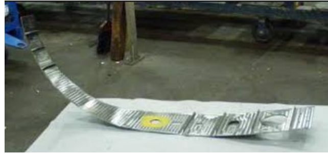
Figure 2-4: (a) Cracking in a cast aluminium ingot due to excessive residual stresses [15], (b) Thin wall-floor aluminium component [45].
