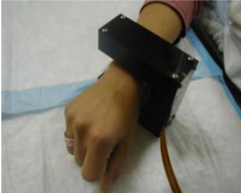
Figure 6.1: Cutaneous beta detector made that can be fixed over the wrist to measure activity input function.[11]
