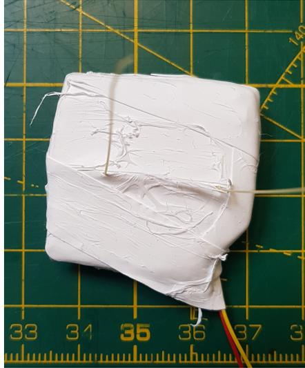
Figure 4.4: Microfluidic detector is wrapped with several layers of PTFE to ensure light photons do not escape out from detector.
