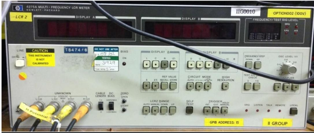
Figure 3.8: LCR meter used for C-V measurement.
