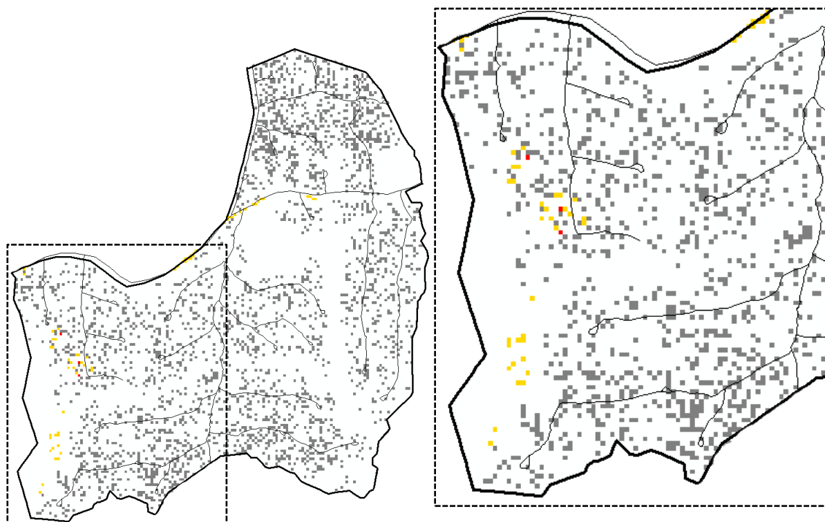
Figure A1.2 Example of a forest management unit in Jamari (logged in 2011) showing the locations of pixels that were logged in grey. CLASlite true and false detections using early Landsat scenes are shown as red and yellow respectively. GPS digitized logging roads are displayed as thin black lines. Pixels that coincided with mapped logging roads were removed from tallies of false detections.
